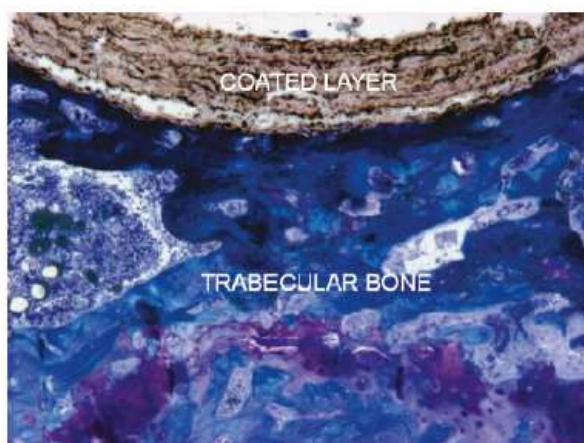
Figure 7. Histological image (5 \times ) of group 3 implant in rat, with toluidine blue coloration showing HA–CNT coating strongly attached to newly grown bone tissues. Normal neobone closed to the coating with normal cell morphology was found.
