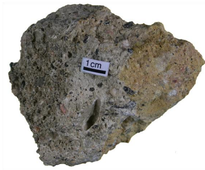
Figure A. 3. Mineralized sample LHU-2 showing the heterogeneous granulometry of the rock, and the yellowish hexavalent uranium minerals.
