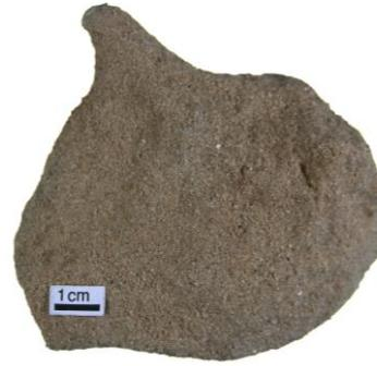
Figure A. 4. Sample LHU-5 corresponding to a relatively well sorted sandstone.
