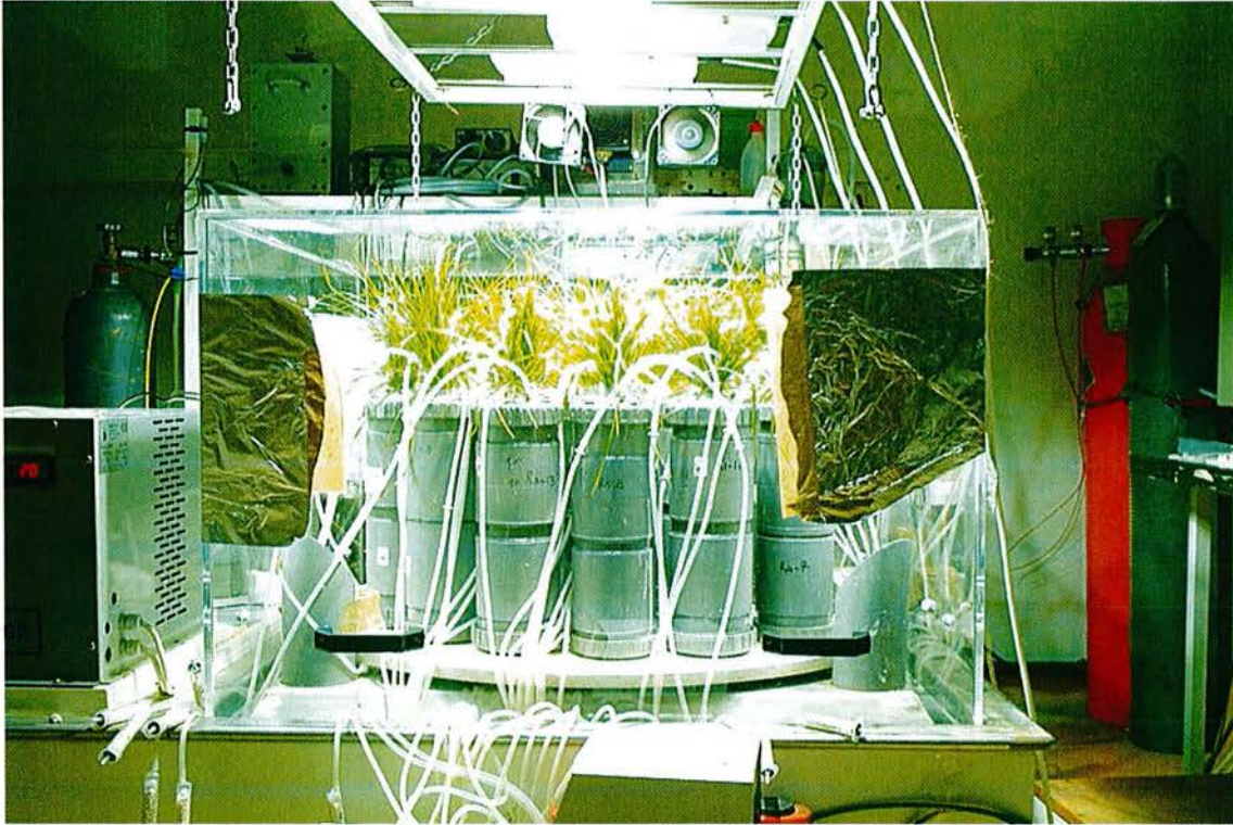
Plate 5.1: Lolium perenne plants in the assimilation chamber during ^{14}\text{C} labelling.
