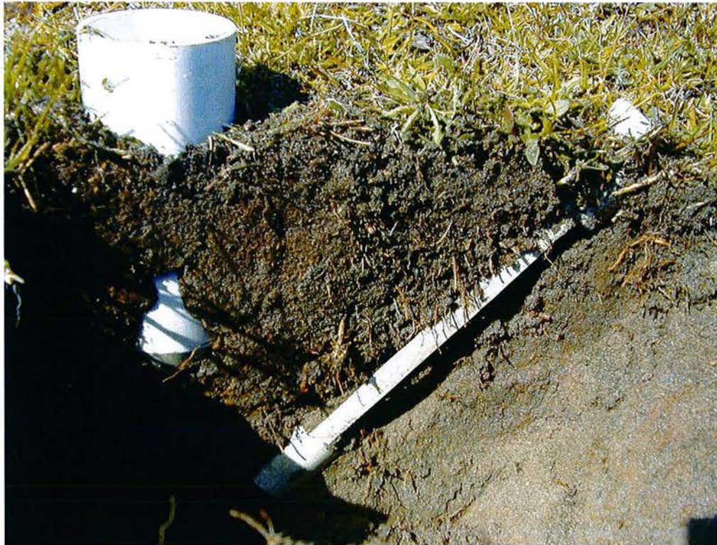
Plate 4.1: View of an “ingrowth core” pipe buried in the field with a 45° angle
