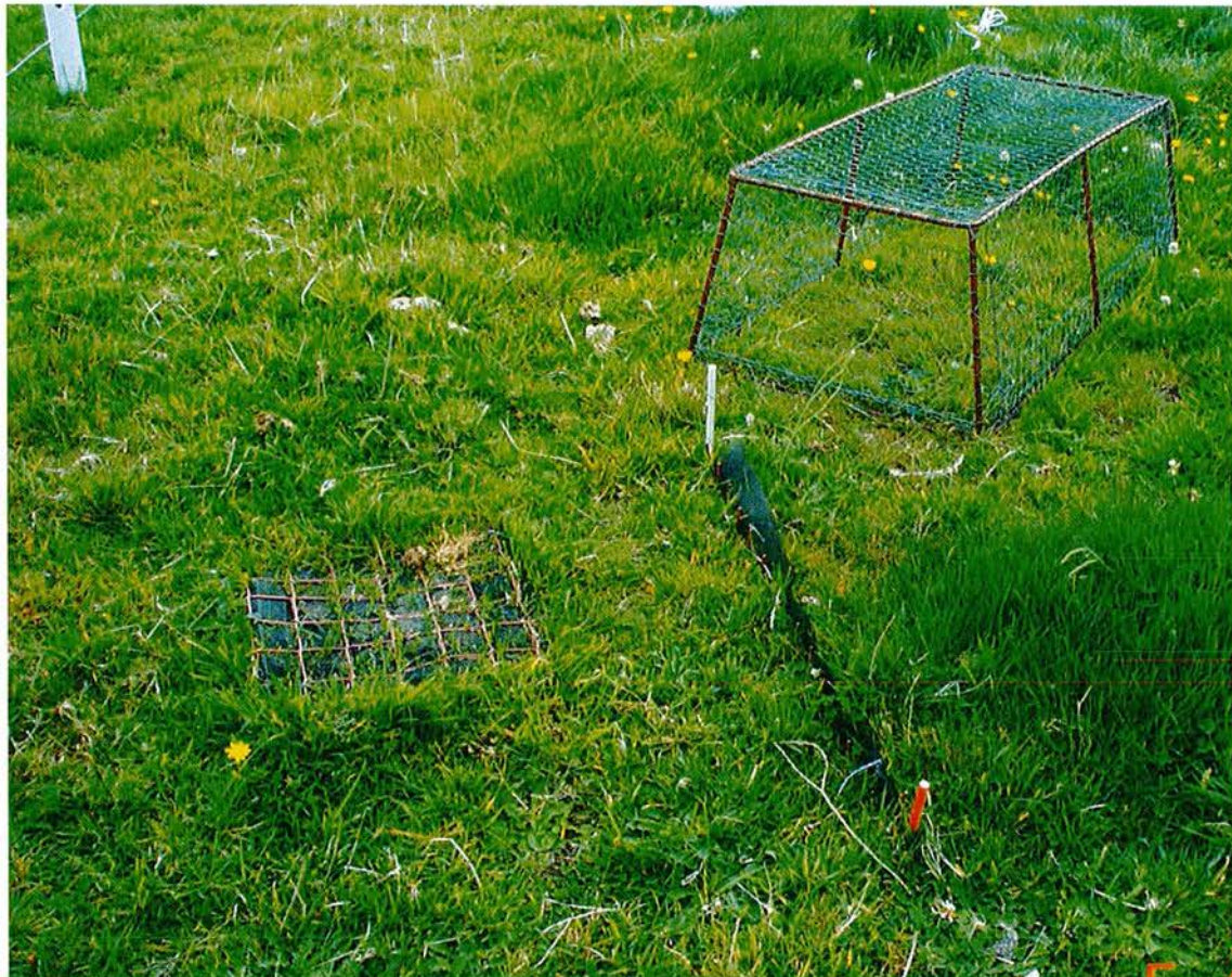
Plate 3.1: Litter incubation bags in the field. Leaf material is placed at the soil surface and root material is buried.
