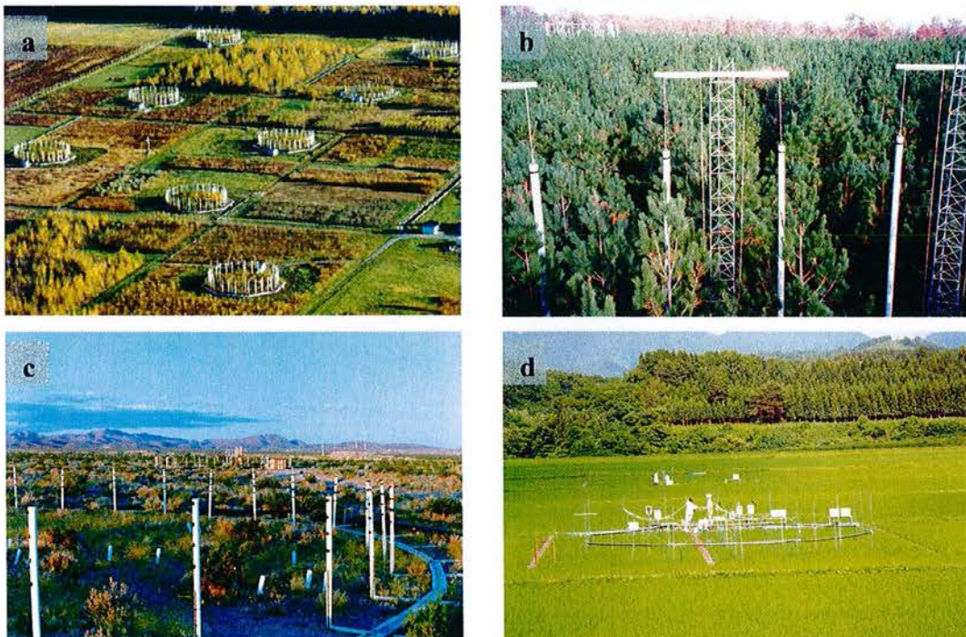
Plate 1.2: FACE systems have been designed to simulate CO 2 enrichment on various ecosystems including (a) an Aspen forest (Wisconsin, USA), (b) a loblolly pine forest (North Carolina, USA), (c) a Mojave desert ecosystem (Nevada, USA) and (d) crops such as rice (Shizukuishi, Japan).
