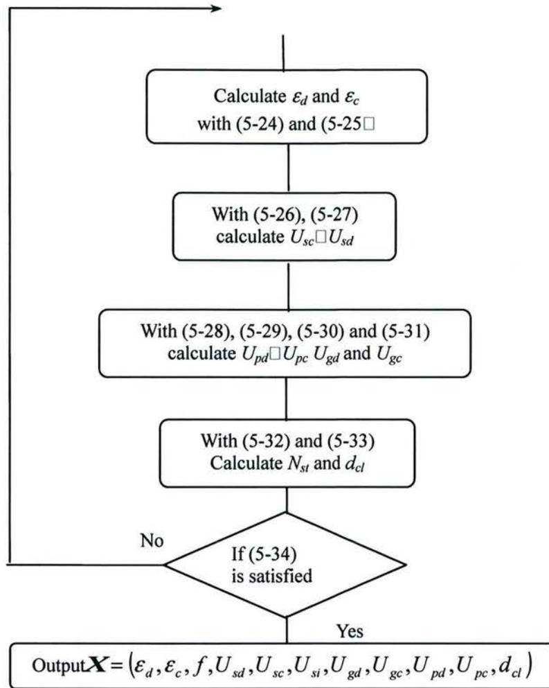
**Fig. 5-3 Calculation Procedure of PFD Model.**
