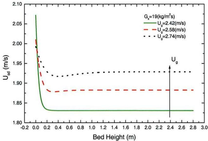
Fig. 5-18  $U_{sd}$  Distribution Along CFB Riser at Different  $U_g$  and  $G_s$
