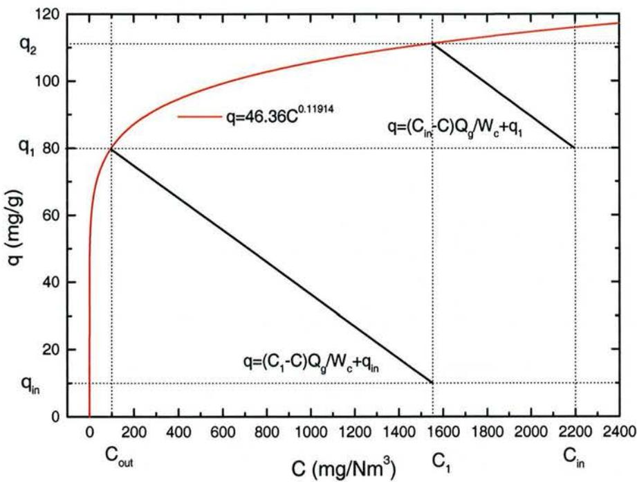
**Fig. 7-9 Operation Lines in Two-stage CFB Adsorber**
