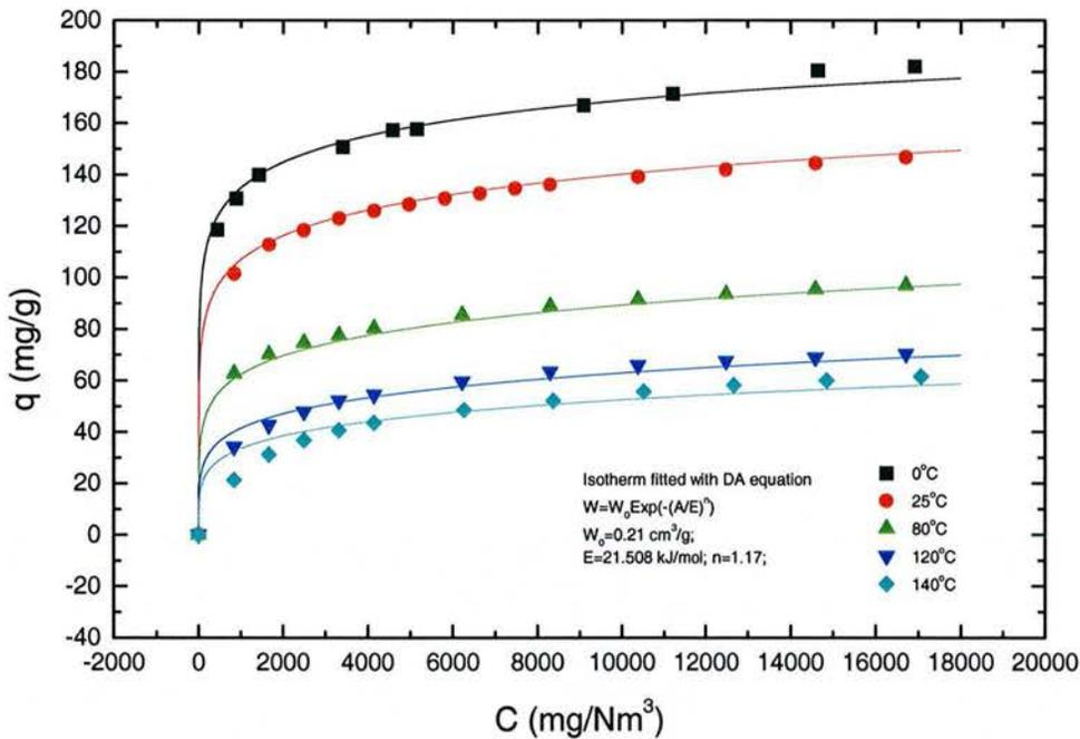
**Fig. 2-11 Test Data Fitted with D-A Equation**
