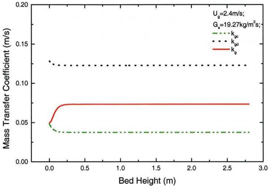
**Fig. 6-4 External Mass Transfer Coefficient in the Bed**
