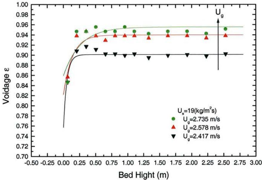
Fig. 5-15 Axial Voidage Distribution for Different  $G_s$  and  $U_g$
