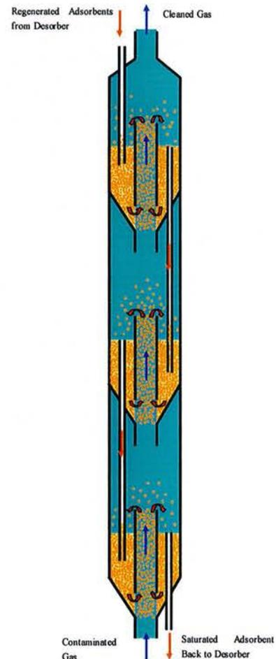
**Fig. 7-8 Multi-stage CFB Adsorber**
