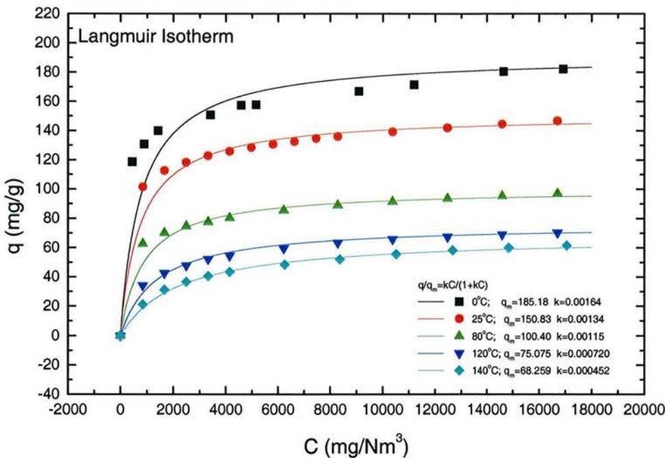
**Fig. 2-7 Test Data Fitted With Langmuir Isotherm**
