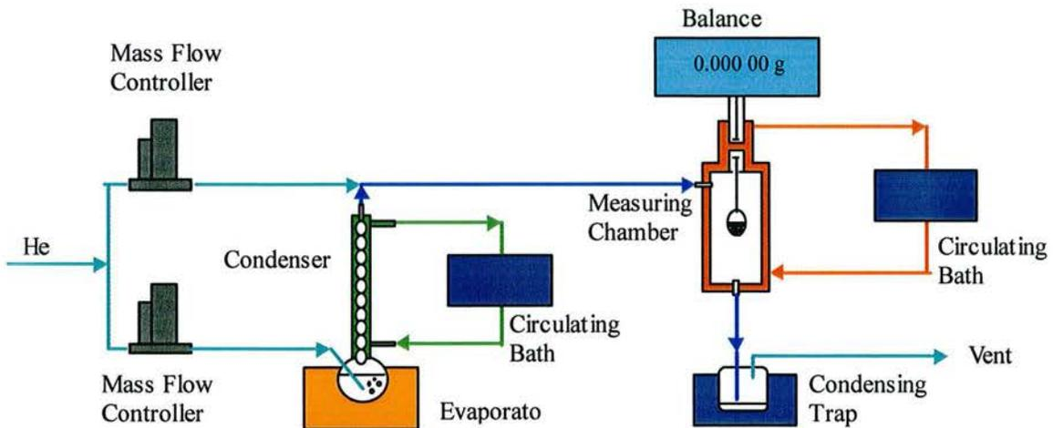
**Fig. 2-2 Isotherm Measurement Setup**
