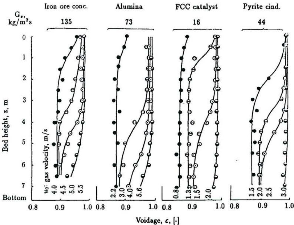
Fig. 5-14 Axial Voidage Distribution
