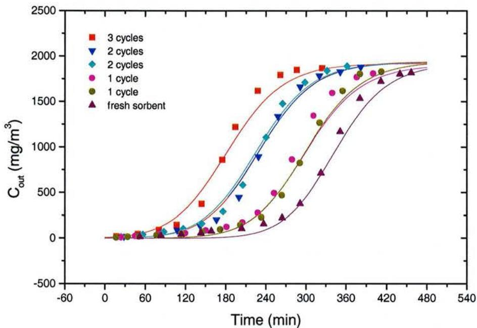
**Fig. 4-5 Exit VOCs Concentrations with Different Fresh and Regenerated Adsorbent**
