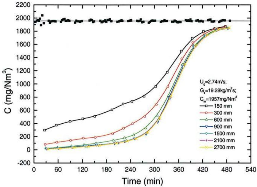
Fig. 3-10 VOCs Concentration Measurements at Different Bed Height
