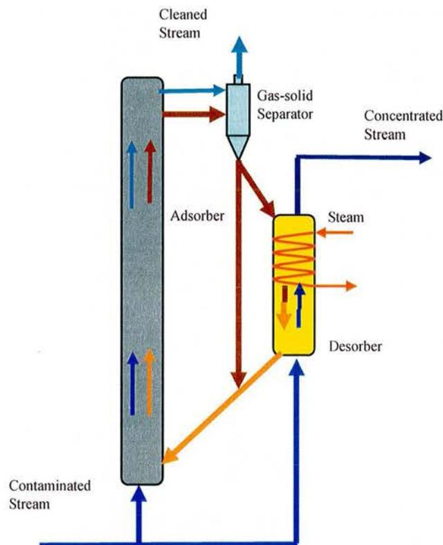
**Fig. 7-1 Schematic Diagram of CFB Adsorption System**
