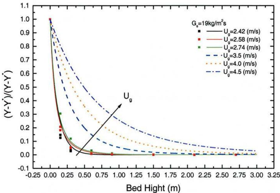
**Fig. 7-4 Residual Concentration Distribution with Different Gas Velocities**
