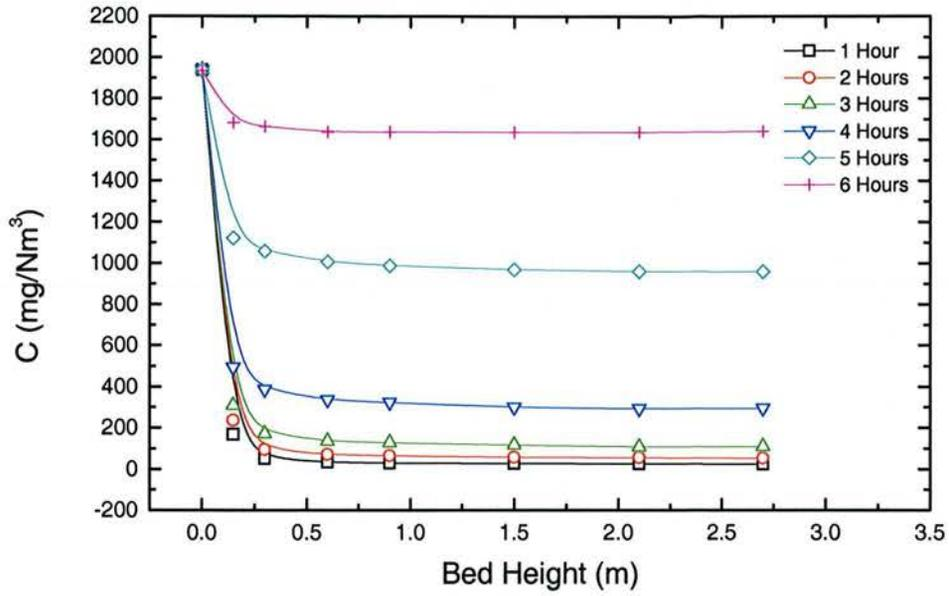
Fig. 3-9 VOCs Concentration Distribution Along CFB Riser
