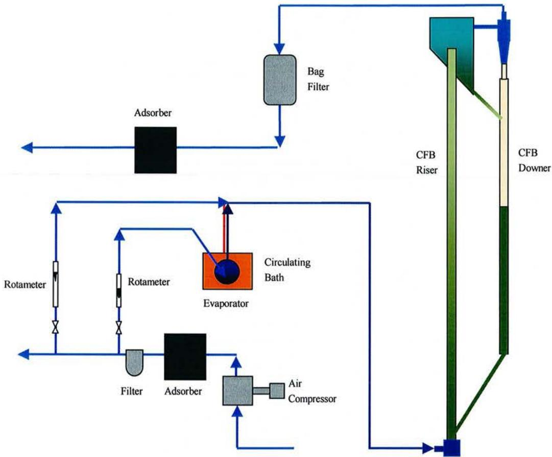
Fig. 3-1 Schematic Diagram of CFB Adsorption experimental setup
