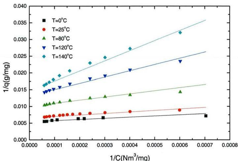
**Fig. 2-5 Experimental data fitted with Langmuir Isotherm**
