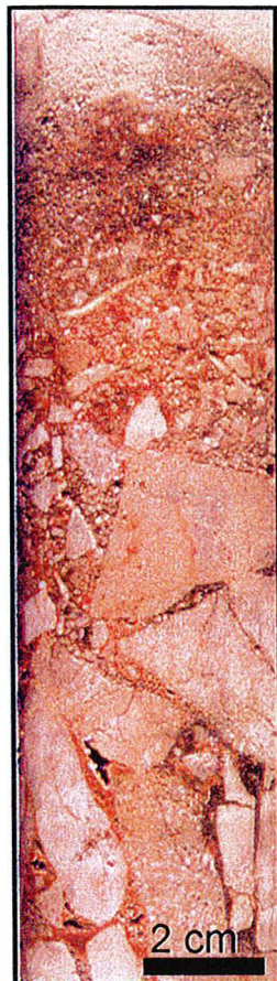
Figure 4. Photograph of a Fe-chlorite solution-collapse breccia at Shea Creek with fragment-supported texture and graded-bedding in the upper part of the breccia.
