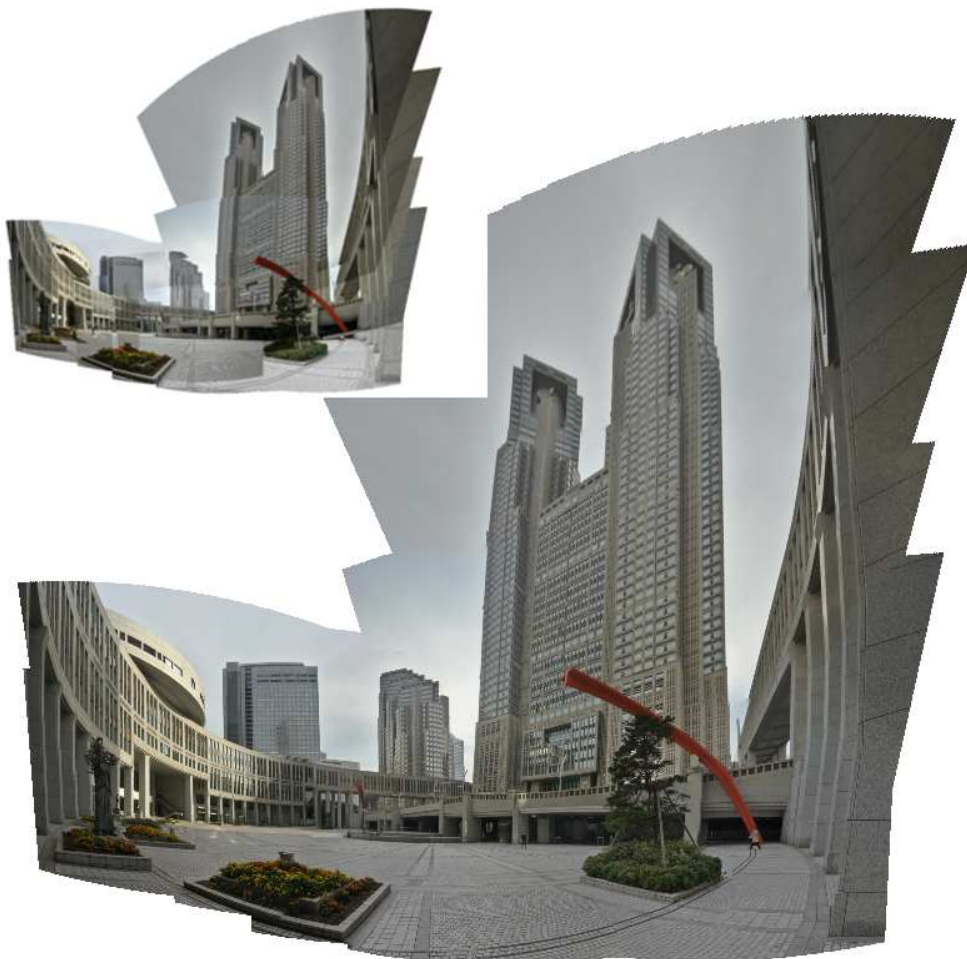
Figure 3.21: Panoramic image composed of a tourist scene using spherical coordinates. Due to the spherical projection model used and the low percentage of image overlap (about 50%), superimposed images are distorted oppositionally (see also Figure 3.22). This complicates the search for seams that align the images in a coherent fashion, and consequently the panoramic image shows slight misalignments. Nonetheless, it is overall visually coherent, especially when compared with a simple successively overwritten map, as shown in small at the top left hand side.
