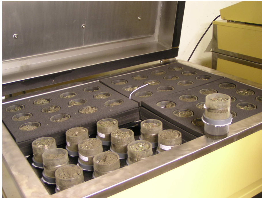
Figure 3.4. MacFadyen extractor used for Collembola extraction in soils with different land uses collected in October 2011 and March 2012, in Naples and surroundings.
