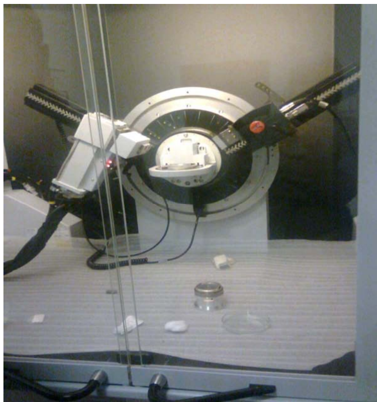
Figure II.13: Dispositif de diffraction des Rayons X.
