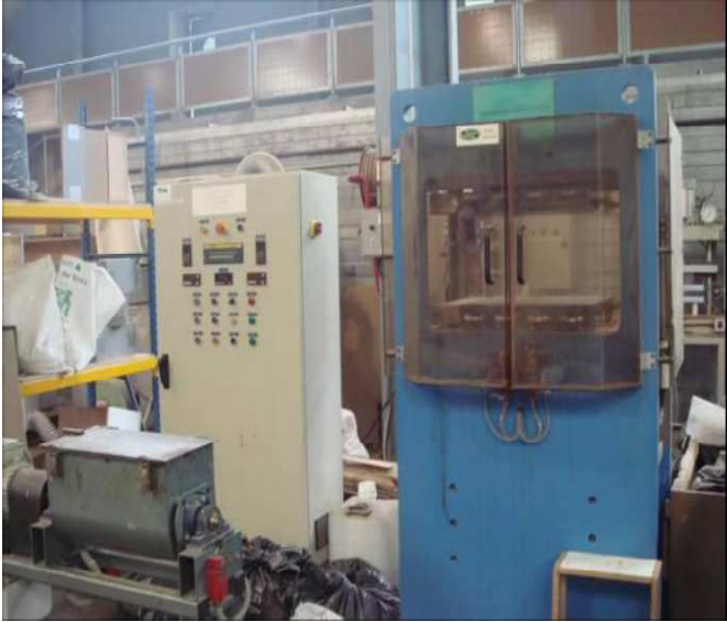
Fig.2. 4 The press system of particleboards
