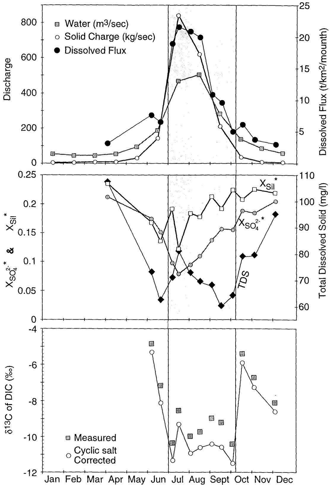
Fig. 7 : Seasonal variation of the water discharge and chemistry of the Trisuli river at Betrawati for TDS, X<sub>SO<sub>4</sub><sup>2-</sup>\*, X<sub>Sil</sub>\* and δ<sup>13</sup>C<sub>DIC</sub>. The shaded area corresponds to the monsoon season. Water discharge data are from the Dept. of Hydrology and Meteorology of Nepal.</sub>
