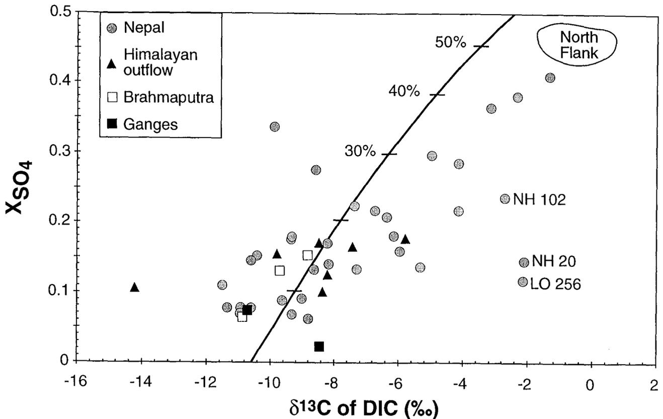
Fig. 6b : Plot of  $\delta^{13}C_{DIC}$  versus  $X_{SO_4}$  for main Himalayan rivers, Ganges and Brahmaputra. The mixing trend corresponds to the alteration by sulphuric acid and biologic carbonic acid of 70% of carbonate and 30% of silicate. Most samples are compatible with a model of alteration driven by soil  $CO_2$  mixed with variable proportion of  $H_2SO_4$ . The 3 labelled samples are close to the MCT, where spring waters are known and may locally influence the TDS.
