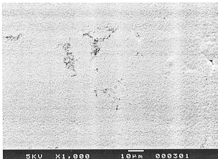
Figure 6.5 j_{\text{appl}} = 159.2 \text{ mA/cm}^2 , \text{Zn(II)-Ni(II)-NH}_4\text{Cl-NH}_3 , \text{pH} = 10 , \text{pNH}_3' = -0.6 , t_{\text{dép}} = 120 \text{ s} , E_{\text{mesuré}} = -1.614 \text{ V/ECS} , \Omega = 1000 \text{ rpm} , T = 25^\circ\text{C} .
