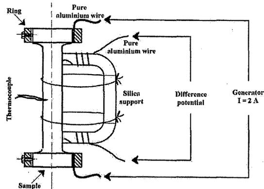
Figure 1: Experimental system for in situ electrical resistivity [9].
