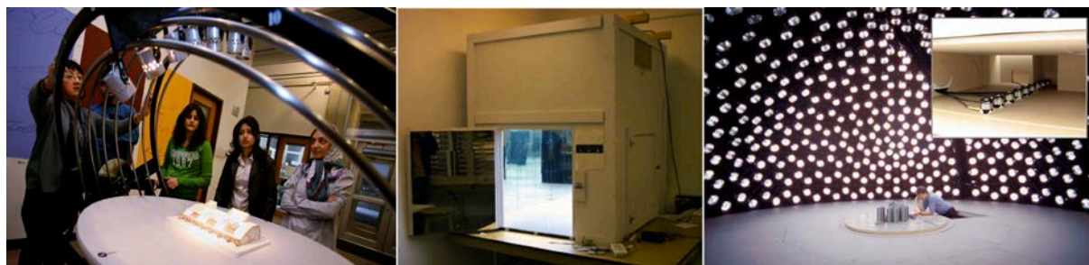
Fig 74. Le Model 126 Heliodon - Texas A&M's College of Architecture / Le ciel artificiel - Université Laval / Le SkyDome - The Welch School of Architecture
