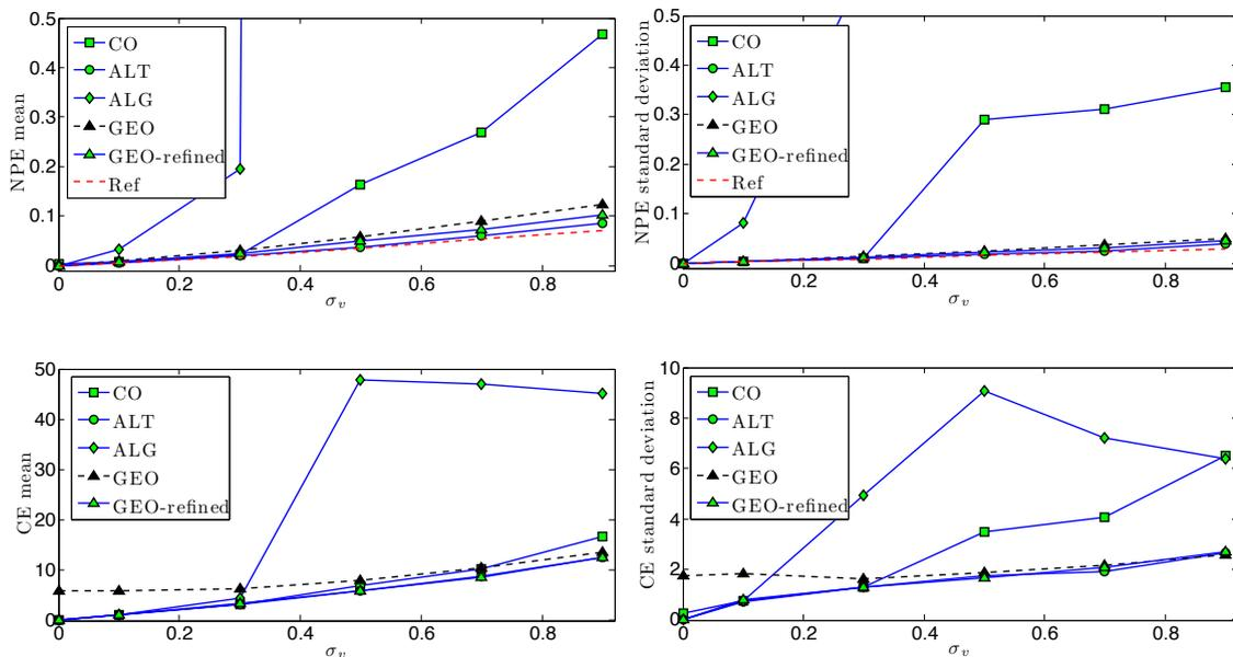
Figure 3.7: System (3.24): parametric error (NPE) (top) and classification error rate (CE) (bottom) versus Gaussian noise standard deviation.
