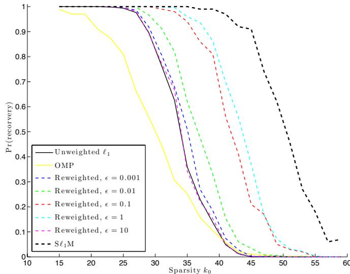
Figure 4.1: Empirical probability of successful recovery versus the sparsity level  $k_0$  for the OMP method [93], the classical reweighting of [25] with various  $\epsilon$ , and the proposed one ( $S\ell_1M$ ).
