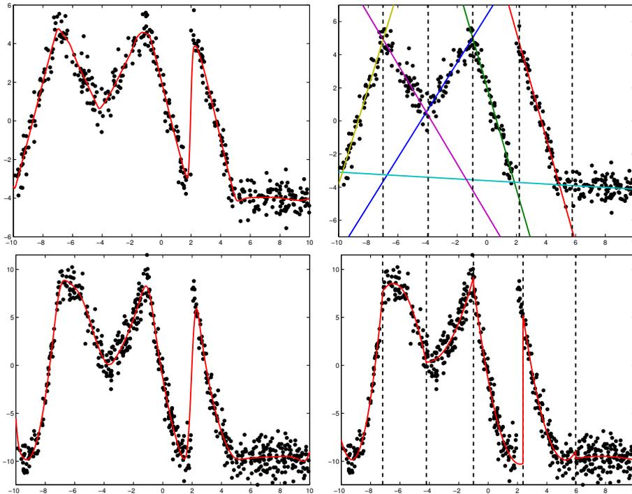
Figure 6.2: Learning a PWA (top) and a PWQ (bottom) model. Left: smooth model obtained after Step 1 of Procedure 12 with  $n=2$  (top) and  $n=3$  (bottom). Right: affine (top) and quadratic (bottom) submodels with the partitions of the input space (dash lines).
