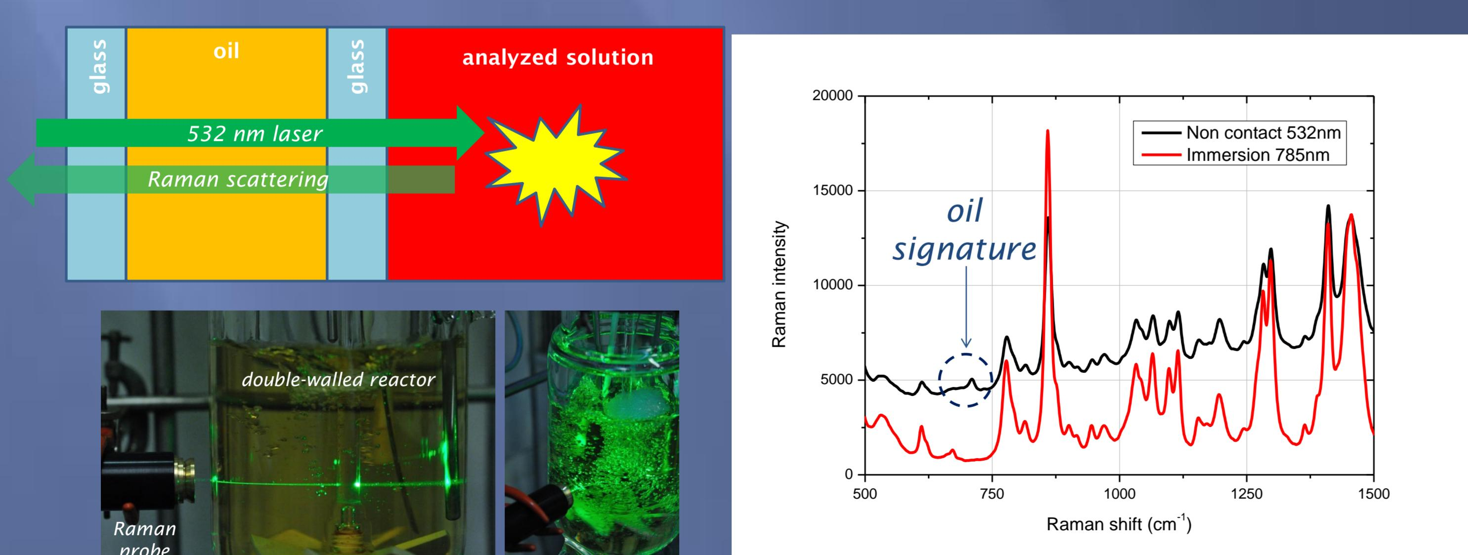
The non-contact probe has given the same spectral signatures as the immersion probe even though the optical beam round-trip through the glass/oil/glass walls. The oil peak in the spectrum at 532nm can be used as the reference for normalization.
