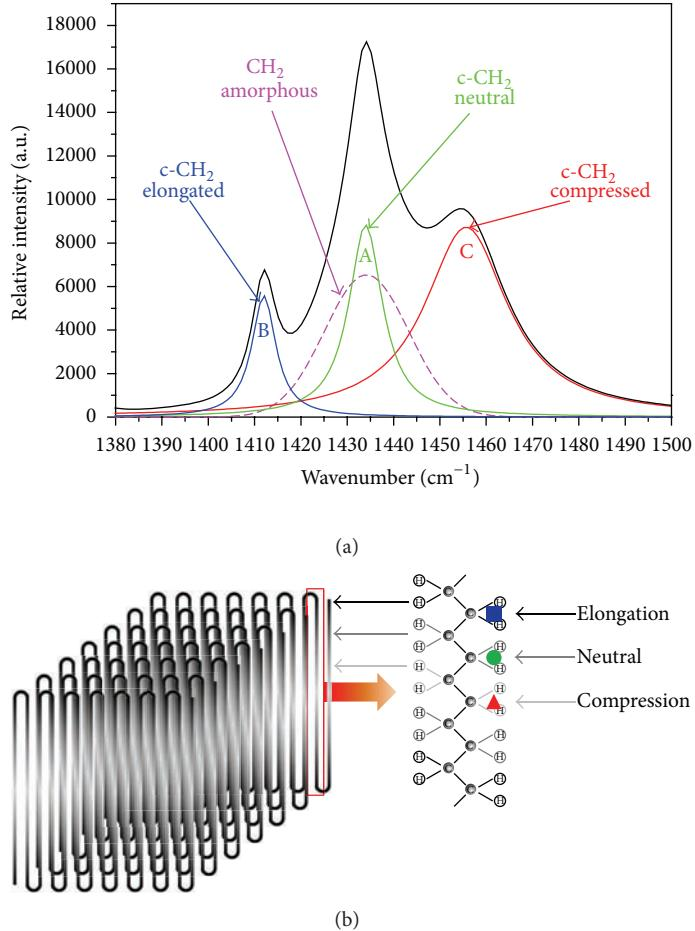
FIGURE 2: (a) Fitting of the LDPE CH<sub>2</sub> spectrum at room temperature with three Lorentzian functions (corresponding to the crystalline phase) and a Gaussian function (corresponding to the amorphous phase); (b) representation of the LDPE lamellar semicrystalline structure.
