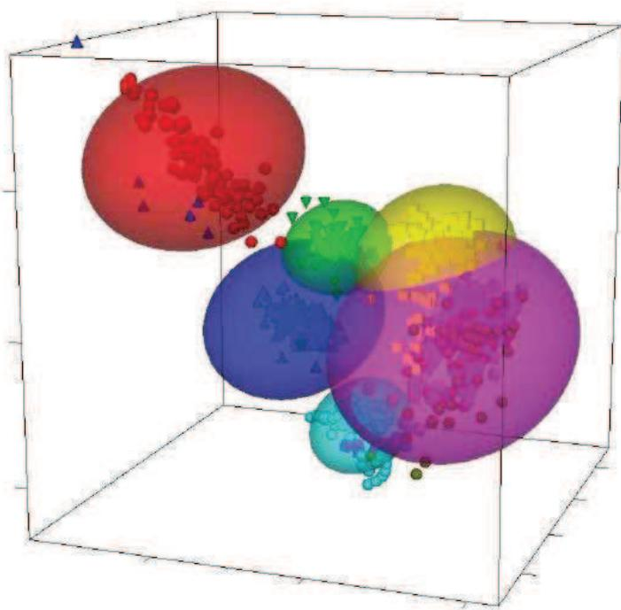
3D diagram of LDPE grades characterization based on PCA and Raman spectroscopy.
