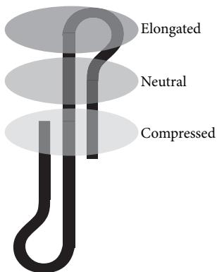
FIGURE 4: Representation of the lamellar crystal structure and position of the three kinds of  $\text{CH}_2$  groups (the black lines represent the C–C skeletal structure;  $\text{CH}_2$  bonds are perpendicular to these lines).
