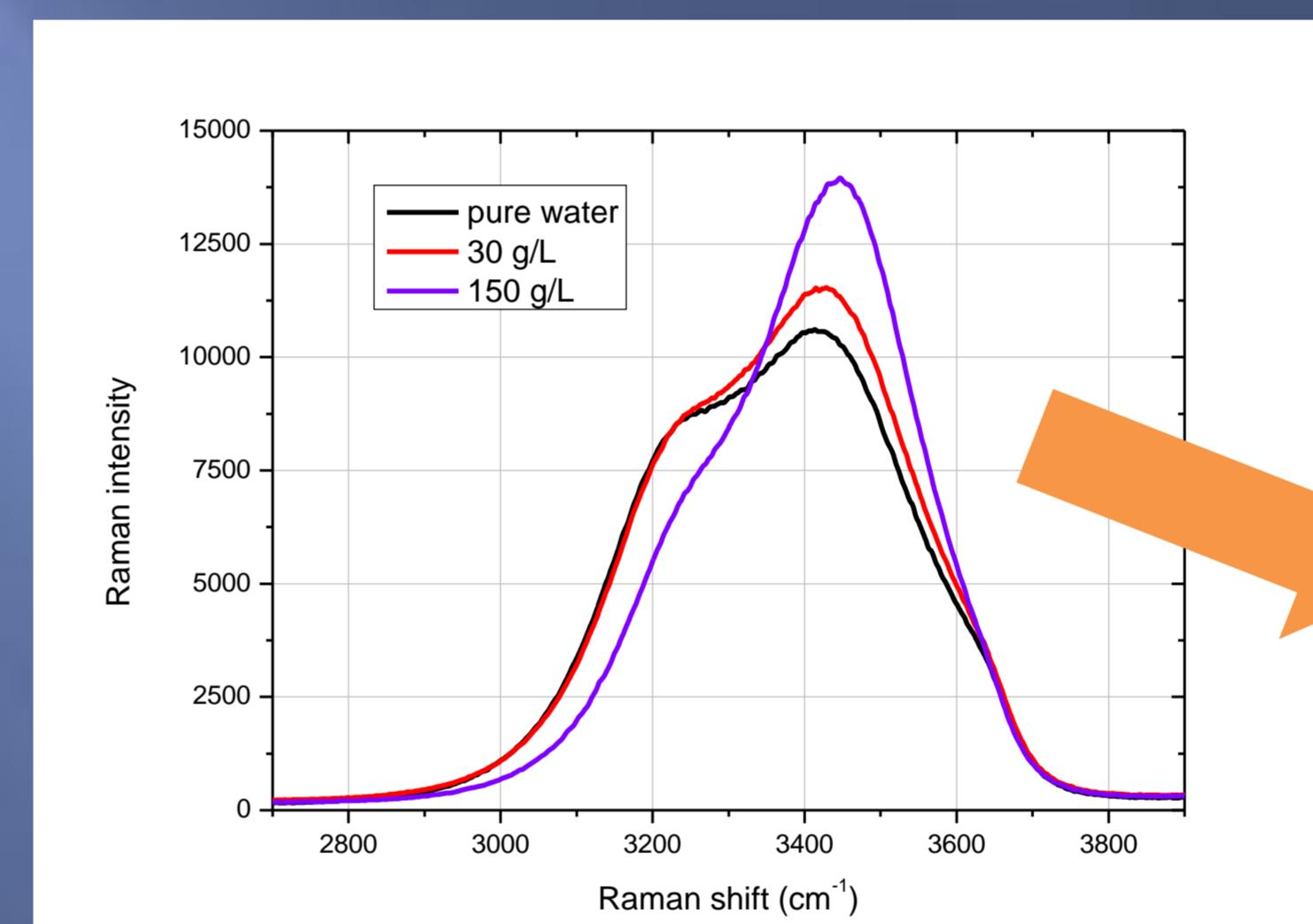
Extraction of a parameter from Raman spectra which is proportional to NaCl concentration
