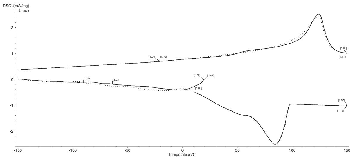
**FIGURE 1.** Complete thermogram of DSC for the grade A: 1<sup>st</sup> cycle (downstroke), 2<sup>nd</sup> cycle (dotted line).
