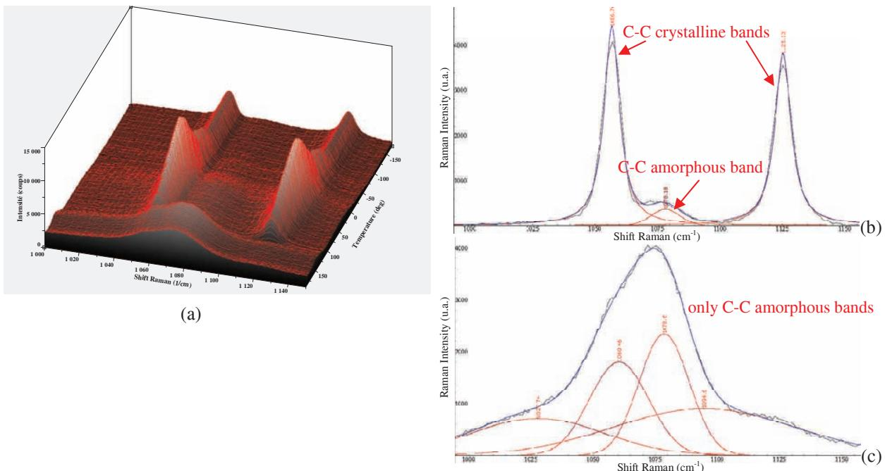
**FIGURE 4.** (a) Temperature mapping (extract) and fitted spectra at  $-170^{\circ}\text{C}$  (b) and  $190^{\circ}\text{C}$  (c) for the grade A.
