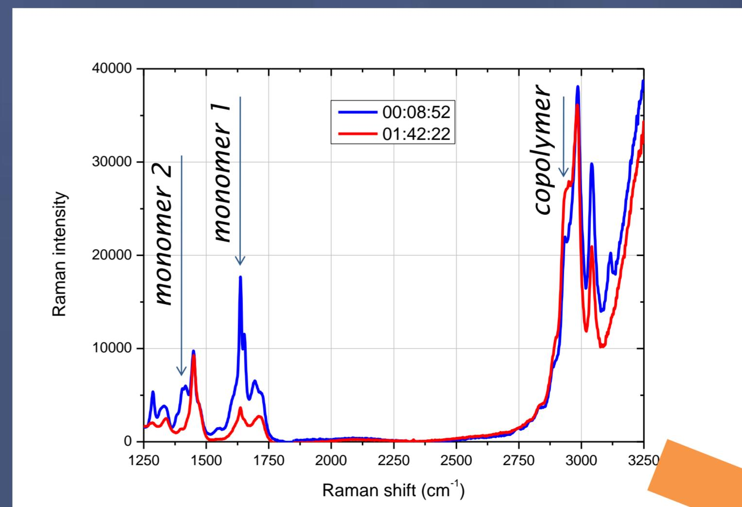
Raman spectra at the beginning and at the end of the copolymerization.
