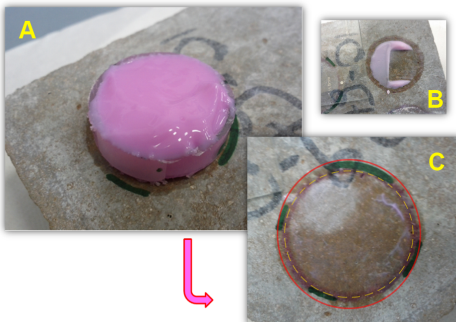
Figure 4.9 – Impregnation test. A: deposit of the gel. B: removal after a fixed impregnation time. C: stain size measurement. A comparison with the stain size obtained for a gel without PAANa is then made.
