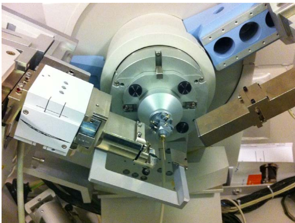
Figure 2.8 The PANalytical X'Pert PRO powder diffractometer at CRM2.
