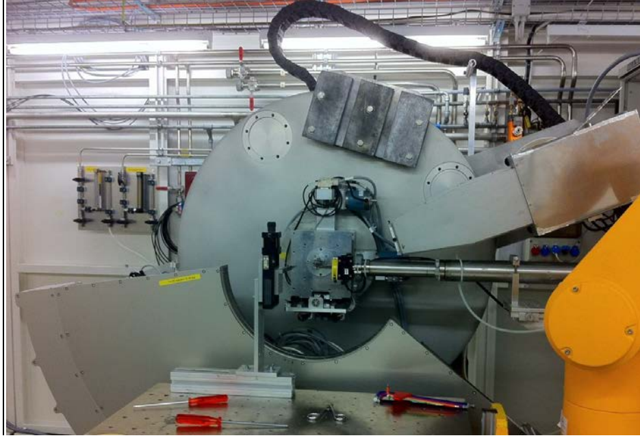
Figure 2.10 The Debye-Scherrer transmission set up on MS-beamline (SLS), Paul Scherrer Institut.
