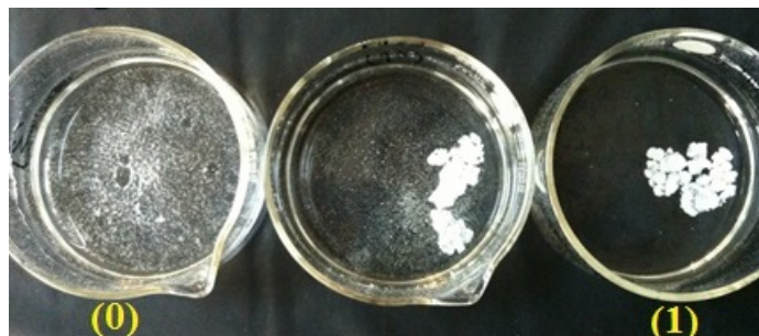
Figure 9: Solid/liquid interaction according to their surface tensions values.
