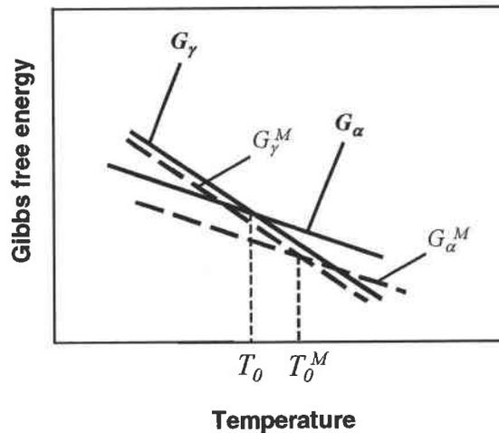
**Figure 1-1** Changing of Gibbs free energy of austenite and martensite with temperature in the case without and with magnetic field,  $\alpha$  – martensite;  $\gamma$  – austenite;  $M$  – magnetic field
