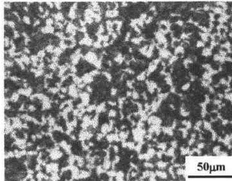
**Figure 5** Microstructure of specimen heated at 880°C for 33min and cooled at 46°C/min with a magnetic field of 14T. (The magnetic field direction and hot-rolling direction are vertical in the picture)
