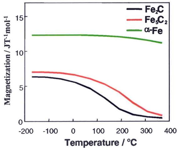
Figure 6 Temperature variations of magnetization of Fe<sub>2</sub>C, Fe<sub>5</sub>C<sub>2</sub> and α-Fe.
