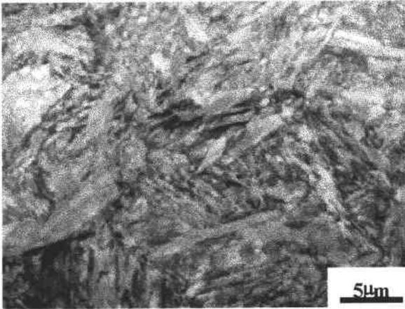
**Figure 2** TEM bright field morphology of martensite obtained by water quenching from 860°C
