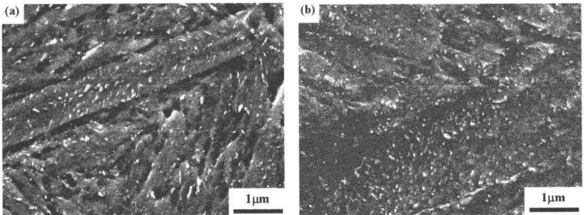
**Figure 3** SEM secondary electron images of carbide precipitates (bright areas) within martensite in specimens tempered at 200°C for 60 min (a) without and (b) with a 14-T magnetic field (the magnetic field direction is vertical in the micrograph).
