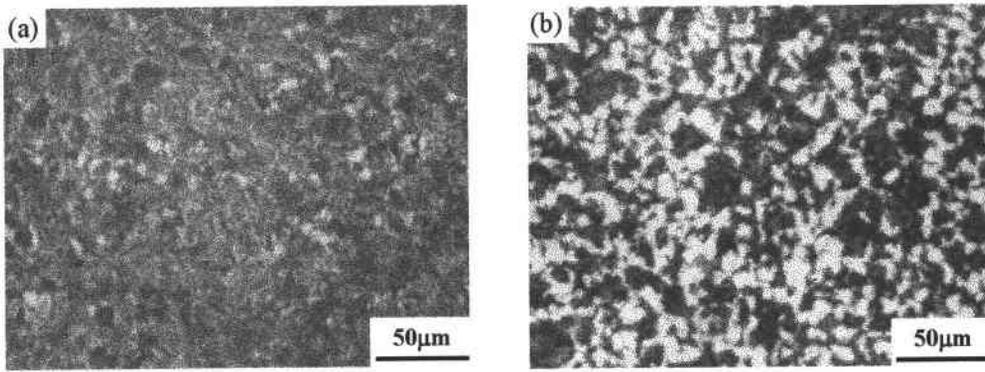
**Figure 3** Microstructure of specimen heat treated at 880°C for 33min and cooled at 46°C/min without (a) and with (b) a 14T-magnetic field, Field direction is vertical in the picture
