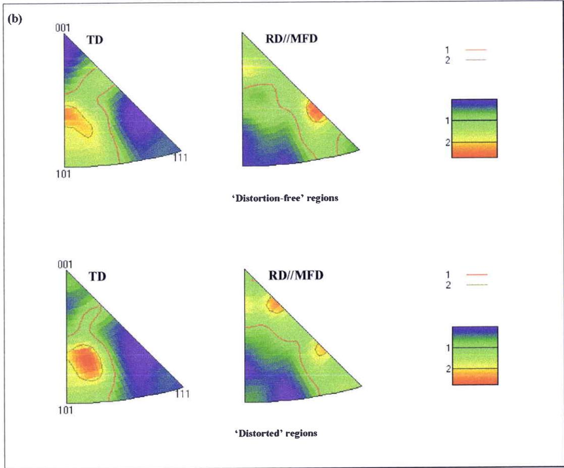
**Figure 10** Transverse direction (TD) and rolling direction (RD//MFD) inverse pole figures of the ‘distortion-free’ and the ‘distorted’ regions obtained by tempering at 650°C for 1 h (a) without and (b) with the magnetic field of 14 T
