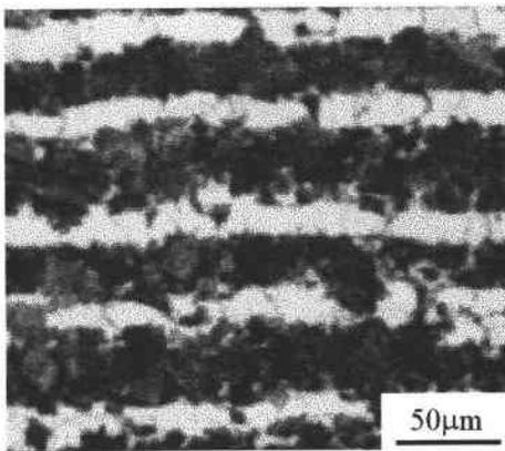
**Figure 1** Banded microstructure in 42CrMo obtained by conventional annealing. Specimens were heated up to 860°C for 30 minutes and cooled inside the furnace at a cooling rate of about 1°C/min (the rolling direction is horizontal in the picture)
