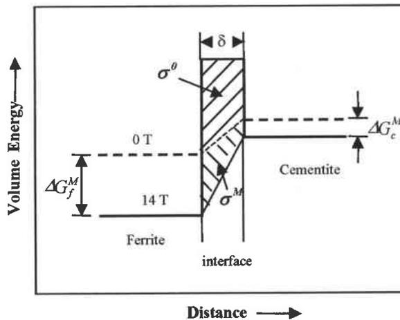
**Figure 12** Schematic illustration of cementite/ferrite interfacial energy without and with the magnetic field
