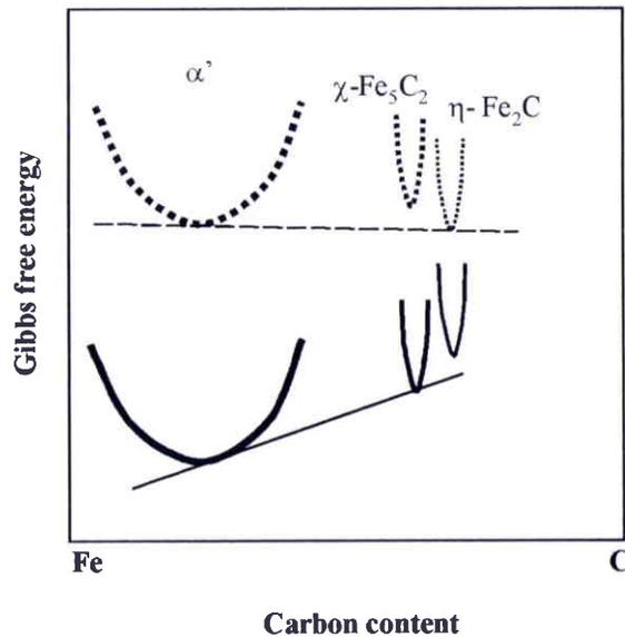
Figure 7 Schematic diagram of Gibbs free energy vs. carbon concentration for  $\alpha'$  martensite,  $\chi$ -Fe<sub>5</sub>C<sub>2</sub> and  $\eta$ -Fe<sub>2</sub>C at 200°C without (dash line) and with (solid line) a 14-T magnetic field.
