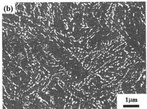
**Figure 4** SEM micrographs of carbides obtained by tempering at 600°C for 1 h (a) without magnetic field; (b) with a magnetic field of 14 T. The field direction is vertical. SEM secondary electron images
