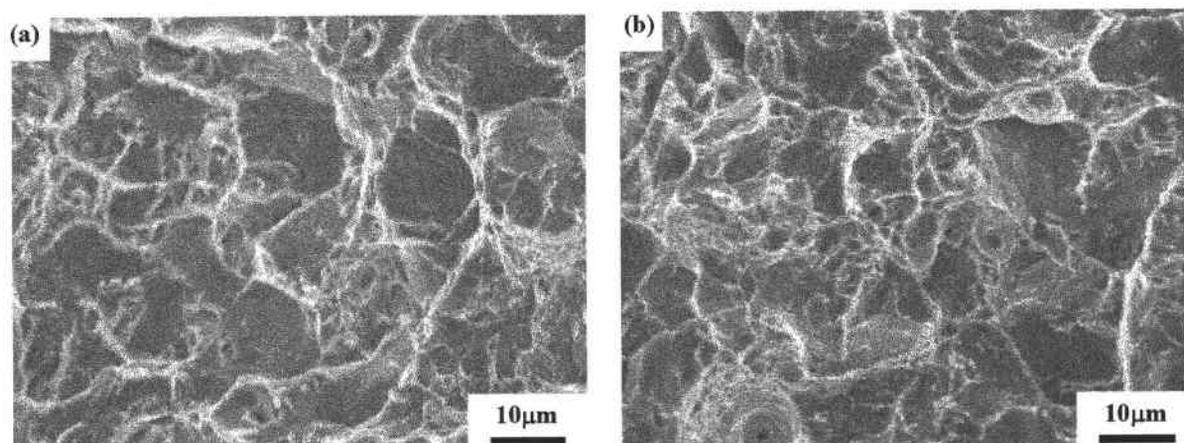
**Figure 5** SEM secondary electron images of impact fractures in specimens tempered at 200°C for 60 min (a) without and (b) with a 14-T magnetic field. The fractographs show the mixture of dimples and intergranular cleavages.
