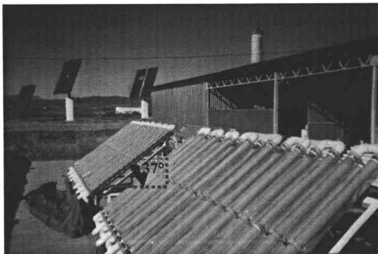
Figure 1.13 CPCs reactor in PSA, volume 190 l
