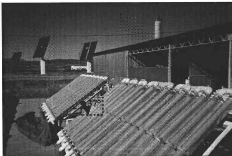
Figure 1.13 CPCs reactor in PSA, volume 190 l
