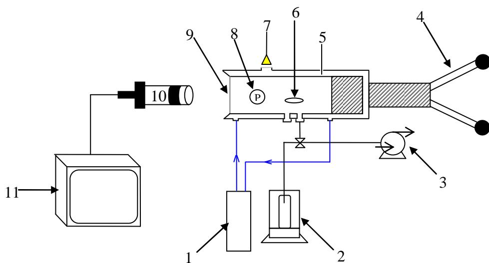
**Figure III-1:** Schema of the VLE apparatus: (1) Thermostated Bath; (2) Analytical Balance; (3) Vacuum Pump; (4) Piston; (5) Temperature Probe (Pt100); (6) Magnetic stirrer; (7) Light source; (8) Calibrated pressure sensor ( $0 < P < 340$  bar); (9) Sapphire window; (10) Video camera; and (11) Monitor.
