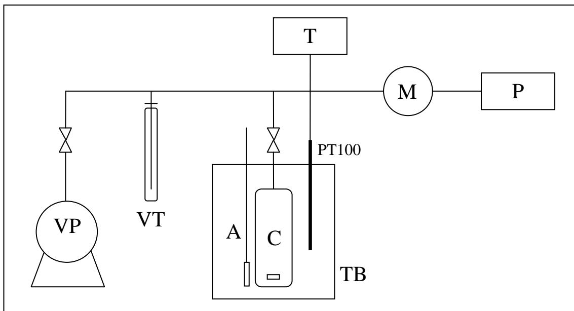
**Figure V-1:** Schema of the VLE apparatus: VP, vacuum pump; VT, vacuum trap; A, magnetic stirrer; C, equilibrium cell; PT-100, platinum resistance thermometer; T, temperature indicator; M, calibrated pressure sensor; P, digital pressure indicator; TB, thermostated bath.
