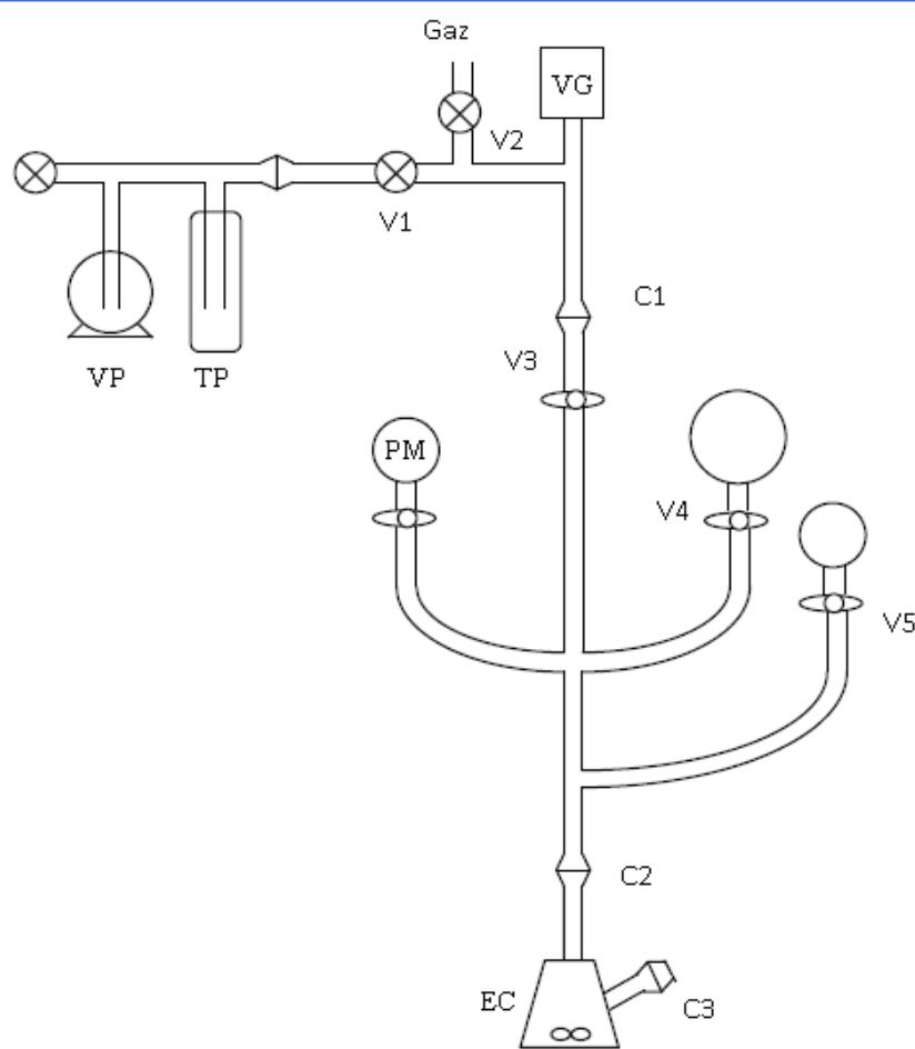
**Figure IV-1:** Schema of the solubility apparatus: VP, vacuum pump; TP, cold trap; VG, vacuum gauge; PM, precision manometer; EC, equilibrium cell; V3, V4, V5, constant volume glass valves; C1, C2, vacuum O'ring connections.
