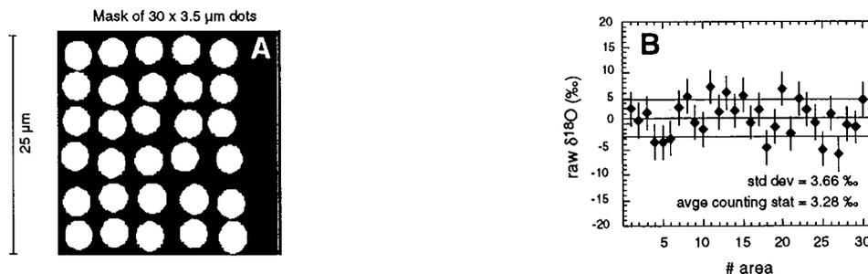
Figure 4. a) Mask used on a polished section of magnetite to investigate the fractionation inside the image plane. b) Variation of raw  $\delta^{18}\text{O}$  inside the image plane for each of the 30 selected areas. The image appears homogeneous in  $\delta^{18}\text{O}$  and the average standard deviation is close to the counting statistics of each point.
