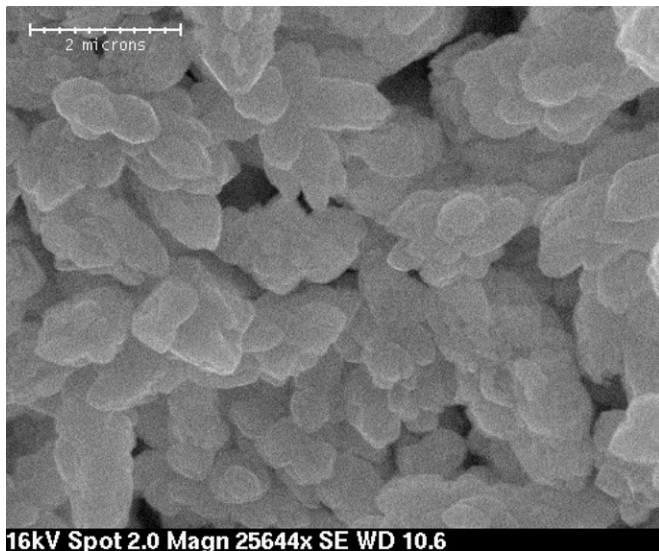
Fig. 3. SEM image of precipitated particles in the reactor/classifier.
