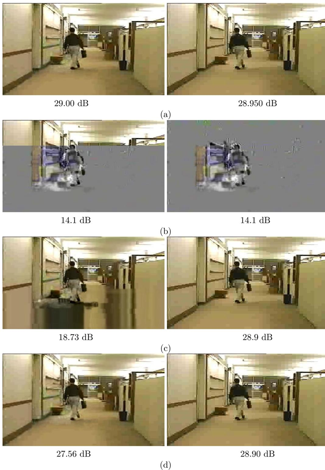
Figure 4.22: Sample of received frames (60 and 61) from the first clip : (a) Reference, (b) DD, (c) PC and (d) ELPC
