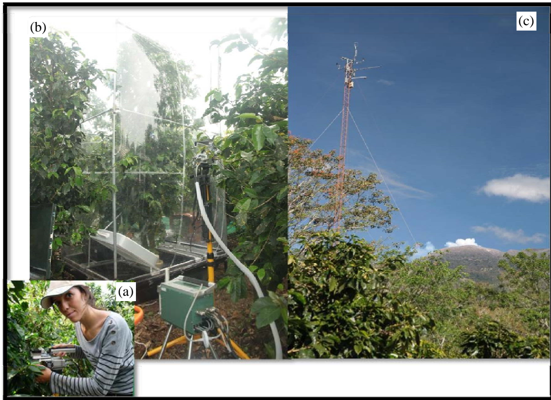
Fig. 12 - Leaf, plant and plot scale measurements of carbon and water exchanges in a coffee AFS in Turrialba, Costa Rica. Leaf gas exchange (a) parameters are used for model parameterization while whole-plant chamber (b) and eddy-covariance (c) are used respectively for intra-plot and plot verification of model predicted fluxes.
