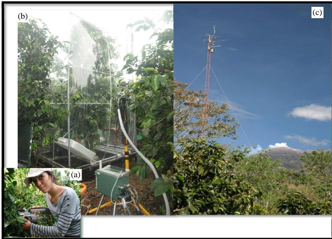
**Fig. 12** - Leaf, plant and plot scale measurements of carbon and water exchanges in a coffee AFS in Turrialba, Costa Rica. Leaf gas exchange (a) parameters are used for model parameterization while whole-plant chamber (b) and eddy-covariance (c) are used respectively for intra-plot and plot verification of model predicted fluxes.
