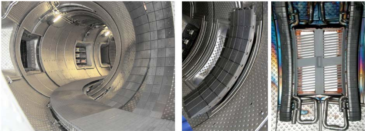
Figure 2.5: Toroidal pumped limiter of the Tore Supra tokamak placed at the bottom of the chamber (left) and modular limiter placed at the midplane (right).
