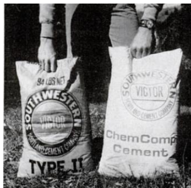
Shrink-comp, in the bag on right, expands on setting, preventing shrinkage cracks common with type II portland cement (left).
