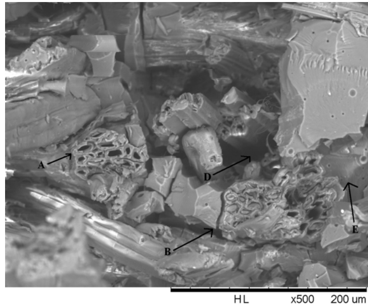
Figure 31 Facies de rupture KENAF T
