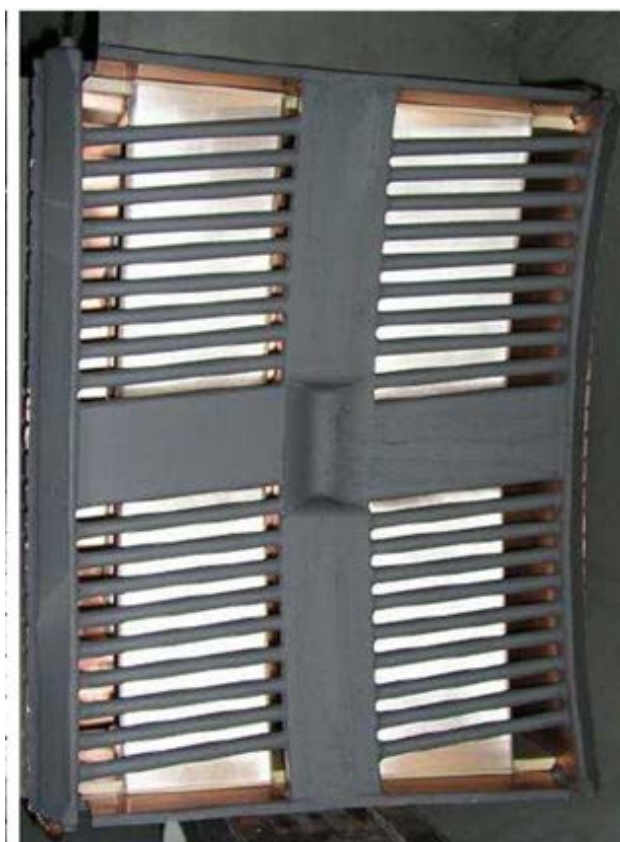
Figure 2.11: Front face of the ILP antenna with the massive poloidal septum and its Faraday screen.
