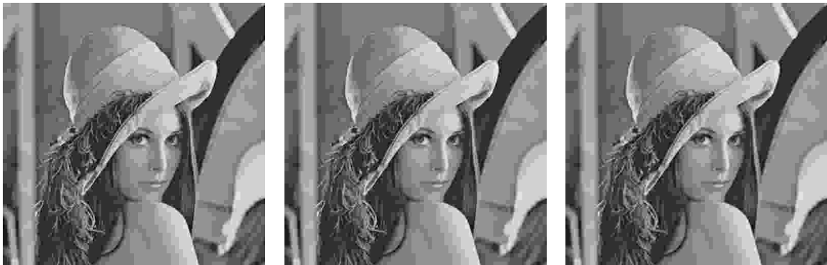
(a) Lena (JPEG), PSNR = 27,33 dB, PSNR - HVS = 23,9 dB, MS - SSIM = 0,74 (b) Lena ( k = 4 ), PSNR = 27,32 dB, PSNR - HVS = 23,89 dB, MS - SSIM = 0,74 (c) Lena ( k = 3 ), PSNR = 27,19 dB, PSNR - HVS = 23,77 dB, MS - SSIM = 0,73
