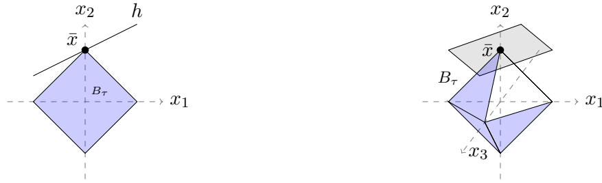
Figure 2.1: Left: Minimum l_1 solution of Ax = h for M = 2 . Right: Geometry of l_1 minimization for M = 3 .
