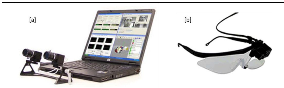
FIGURE 54. Systèmes d'eyetracking [a] fixe (FaceLab) [b] mobile (Mobil'eye)
