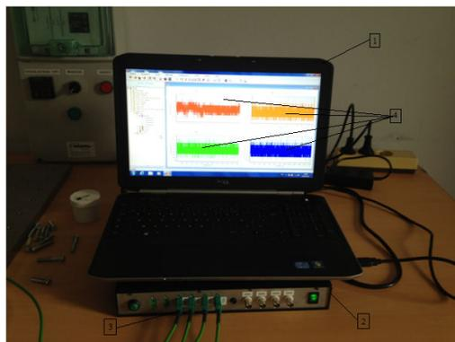
*Figure.V.12. Kit d'acquisition.*
