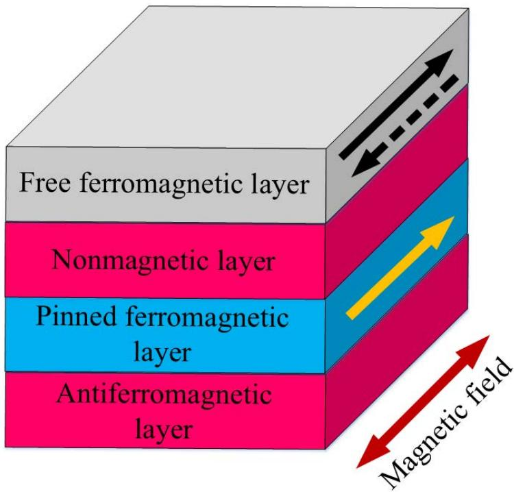
Figure 1.8 The structure of a spin-valve system.
