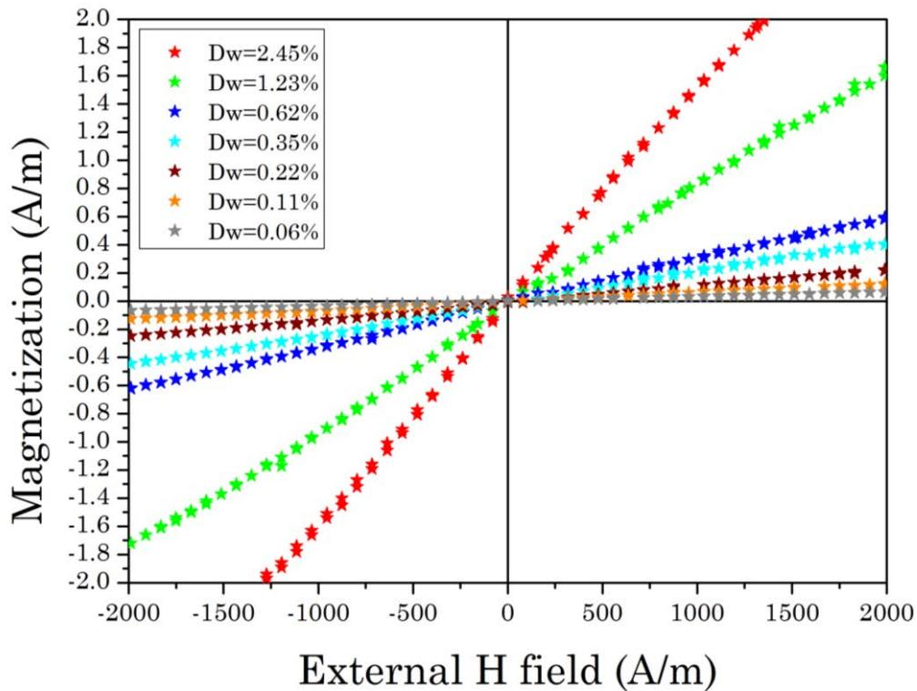
Figure 3.22 The hysteresis curves of fluid MAG-D's concentrations.
