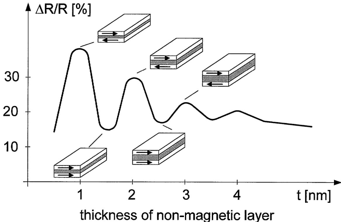
Figure 1.2 Evidence of oscillatory exchange coupling in thin film multilayers [3].
