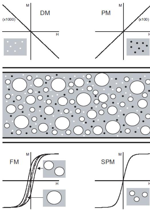
*Figure 1.23 The schematic dependence of ferromagnetic particles injected into a blood vessel as function of their size. The biomaterials in the blood vessel are diamagnetic (DM) or paramagnetic (PM). The injected particles can be ferromagnetic (FM) or superparamagnetic (SPM) [46].*
