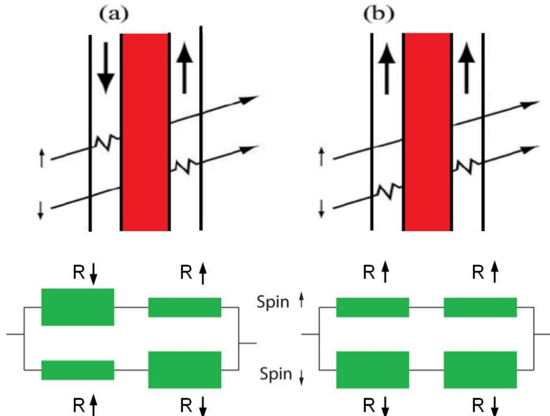
Figure 1.6 Schematic of giant magnetoresistance in a multilayer, two magnetic layers are polarized in the opposite directions (a) or in the same direction (b).
