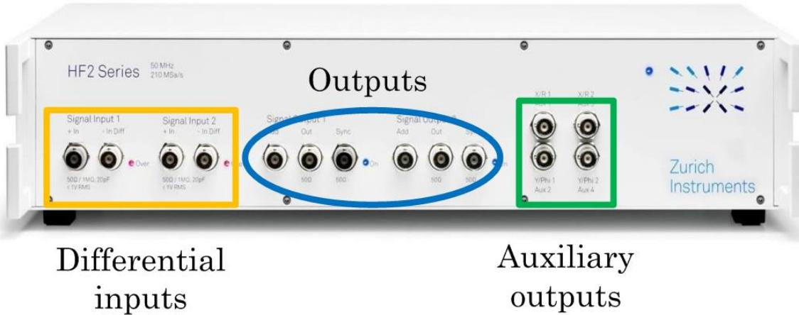
Figure 2.22 The schematic of the HF2IS Impedance Spectrometer.
