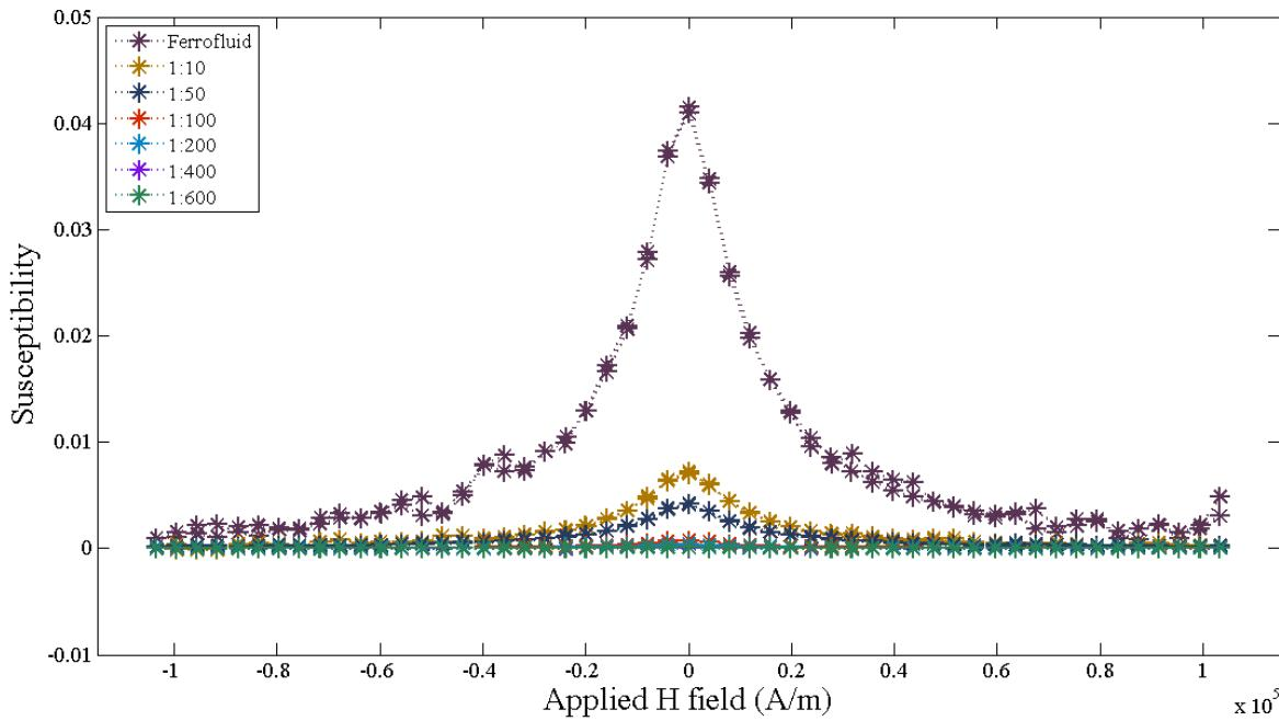
Figure 3.14 Initial magnetic susceptibility  $\chi_i$  as a function of an applied field (A/m).
