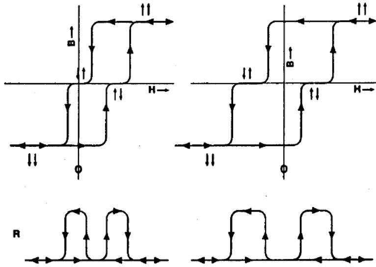
Figure 1.10 Principle of the spin-valve sensor [17].
