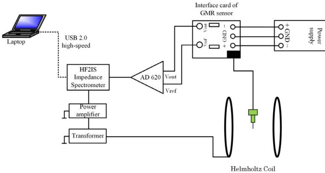
Figure 2.24 Measurement setup of the GMR sensor.
