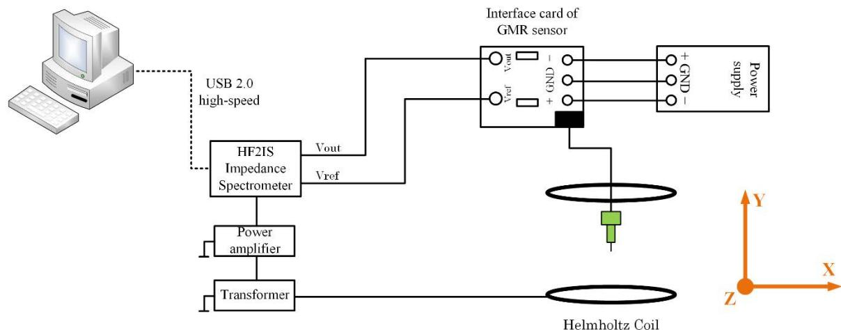
Figure 2.40 Measurement setup to characterize the GMR sensor.
