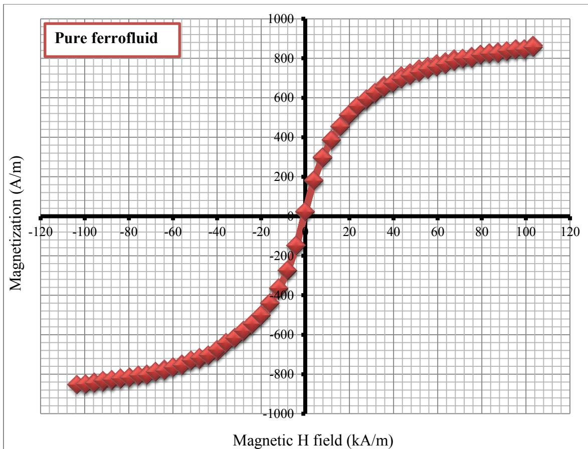
Figure 3.11 Magnetic hysteresis curve of pure ferrofluid.
