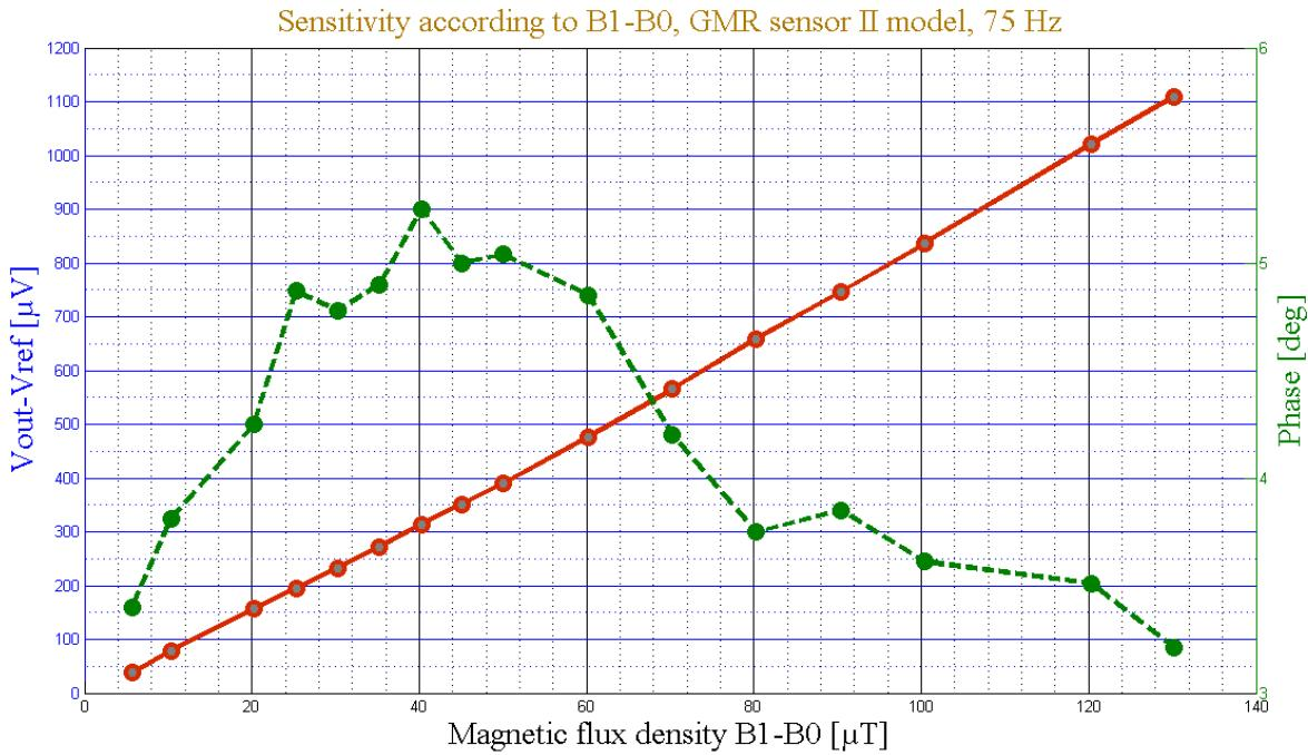
Figure 2.44 The output voltage results obtained by the probe GMR sensor ( $\mu$ V) and phase calculation (deg) with one resistor ( $2.128 \text{ k}\Omega$ ) as a function of the changes in magnetic flux density ( $\mu$ T).
