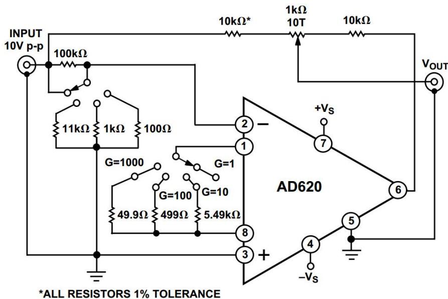
Figure 2.16 The pins schematic of the AD 620 [70].
