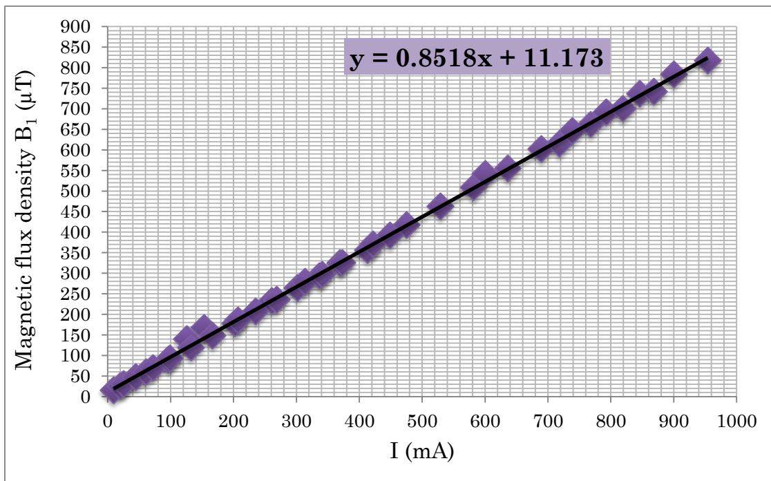
Figure 2.34 Measurement the magnetic flux density  $B_1$  ( $\mu$ T) as a function of the input current (mA) applied to 60 Hz.
