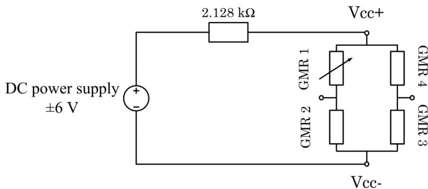
Figure 2.42 Power supply circuit with two additional resistors.
