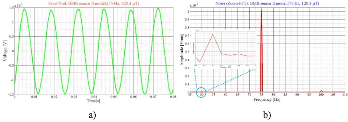
Figure 2.43 The GMR sensor's output voltage ( $V$ ) with  $2.128 \text{ k}\Omega$  (a) and FFT detection from  $V_{out-Vref}$  of the GMR sensor for frequency 75 Hz (b).
