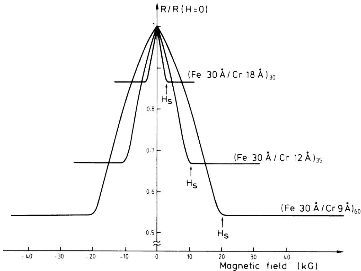
Figure 1.3 Magnetoresistance for several Fe/Cr multilayers at 4.2K [1].
