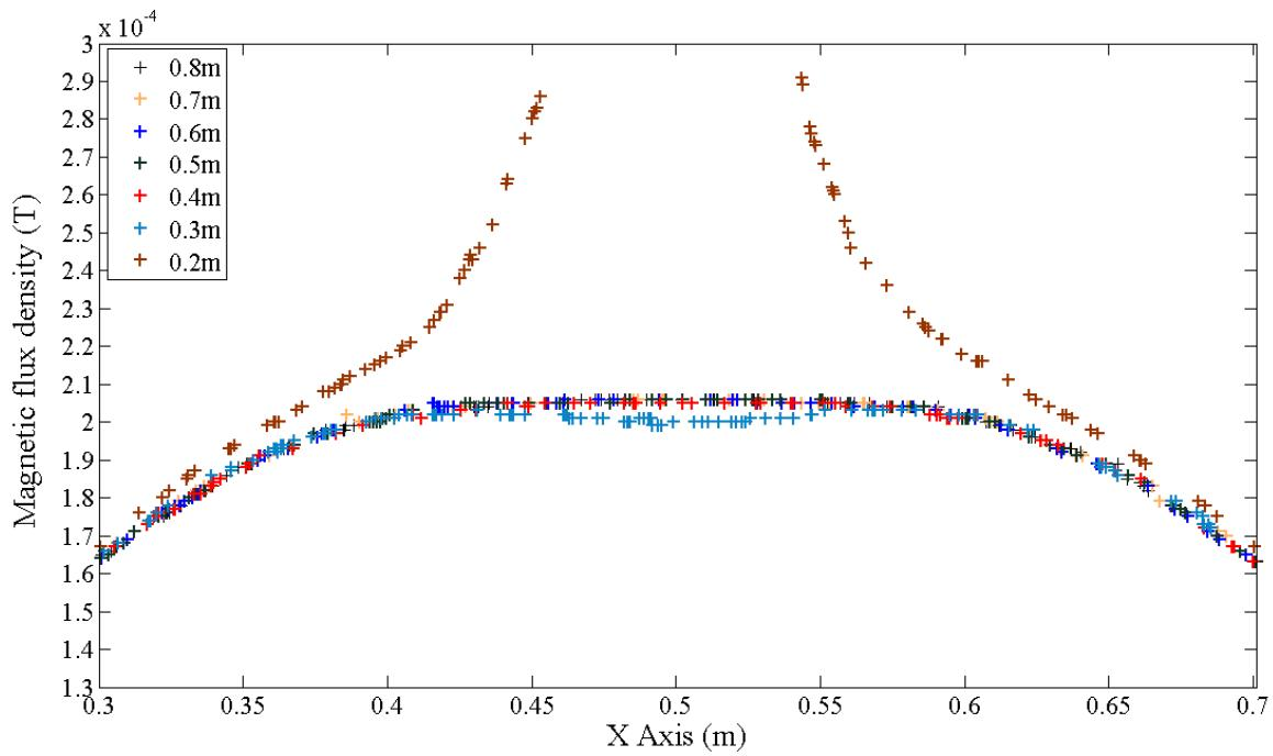
Figure 2.14 Changing the magnetic flux density ( $B$ ) in center of the Helmholtz coil by changing the position of the displacement system along X axis.
