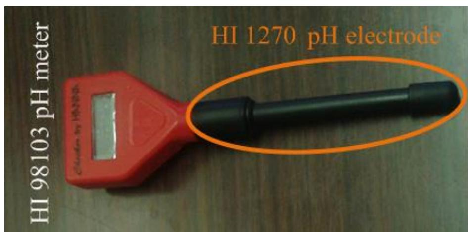
Figure 4.8 The pH meter and its pH electrode.
