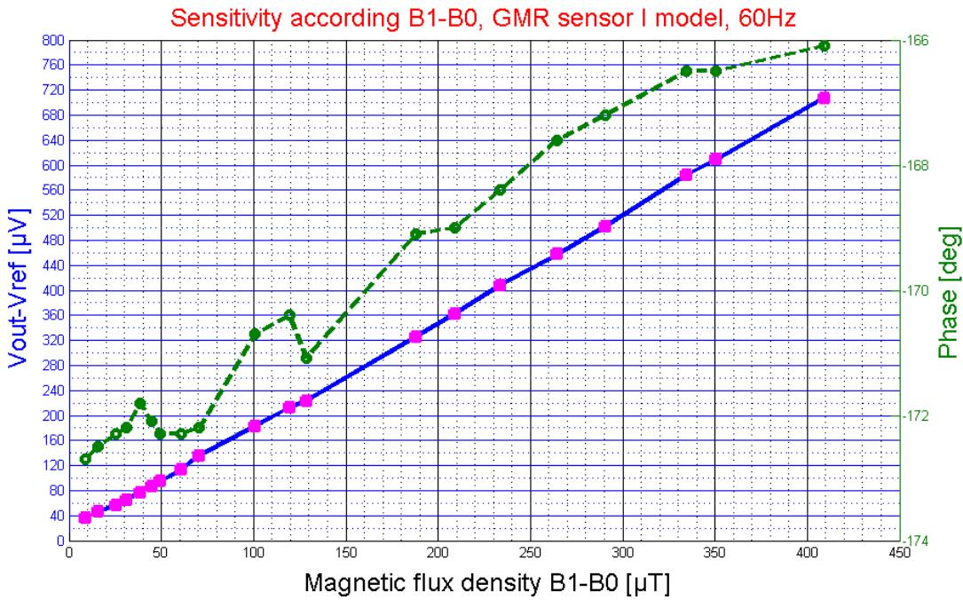
Figure 2.37 Output voltage ( $\mu\text{V}$ ) and phase calculation (deg) with two resistors  $809 \Omega$  as a function of the total changes magnetic flux density  $B_1 - B_0$  ( $\mu\text{T}$ ).
