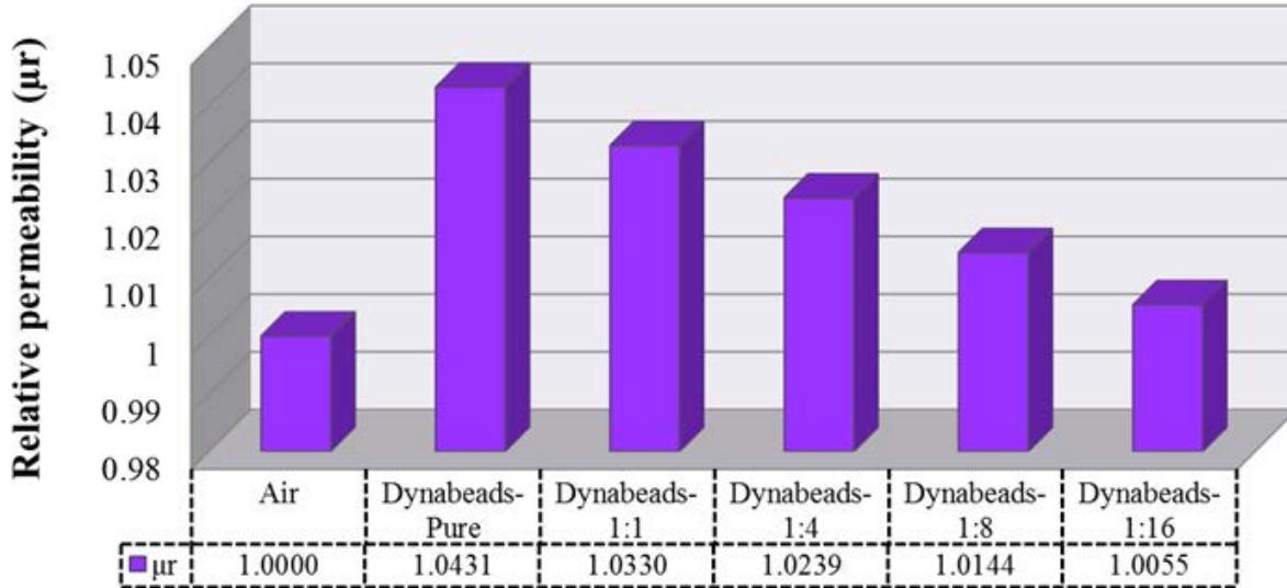
Figure 4.16 Relationship between relative permeability ( $\mu_r$ ) and different magnetic fluid concentrations.
