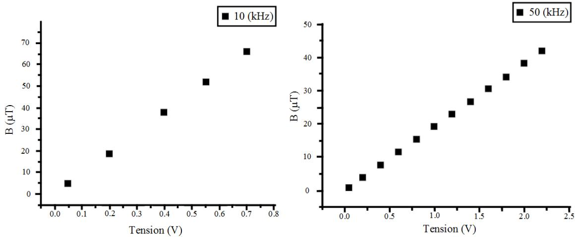
*Figure 2.10 Measurement the magnetic flux density ( $\mu\text{T}$ ) as a function of the input voltage applied to 10 and 50 kHz.*
