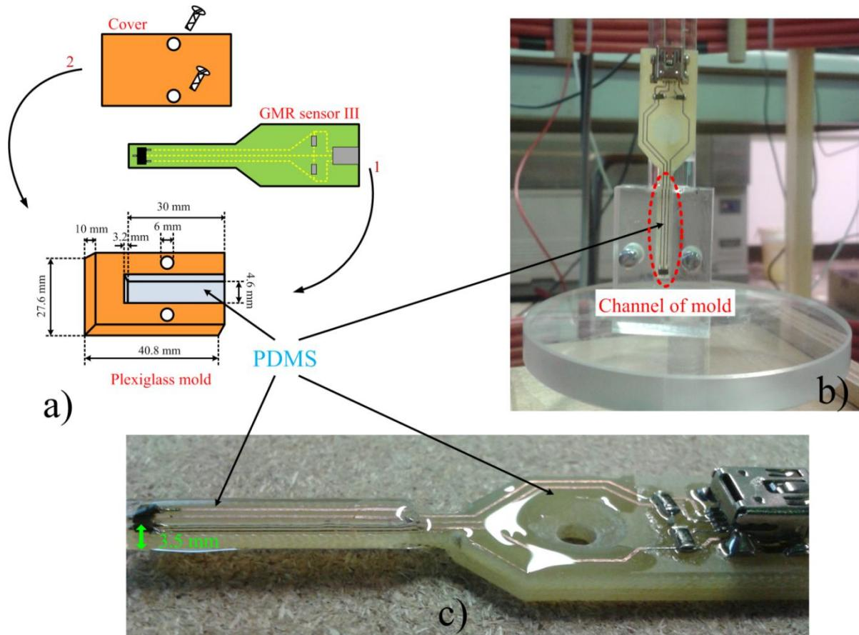
*Figure 4.14 The insulation steps of GMR sensor: preparation of plexiglass mold (a), sensor's positng in the channel of mold (b), GMR sensor III with protective PDMS layers (c).*
