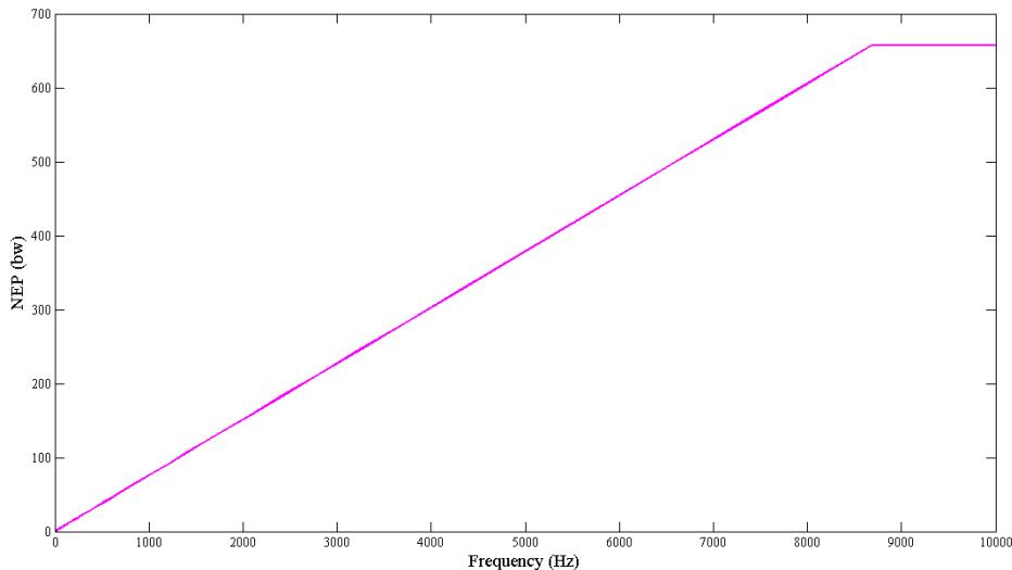
Figure 2.21 Noise equivalent power according to frequency (Hz).
