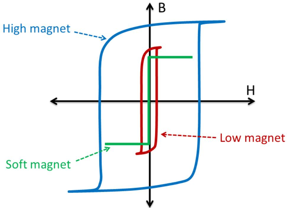
Figure 1.22 Typical Hysteresis curves for hard, low and soft magnetic materials.
