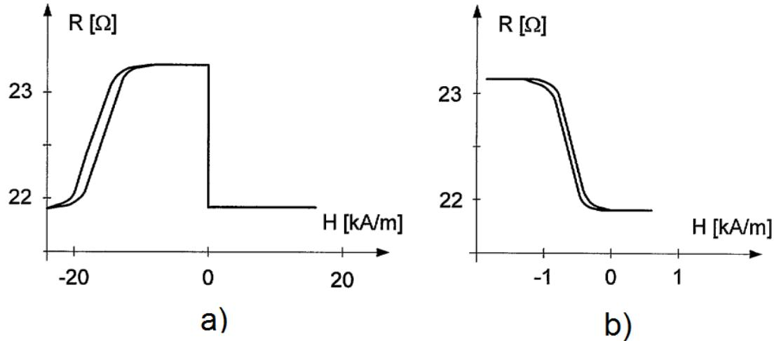
Figure 1.9 Hysteresis loops of the spin valve sensors [14].
