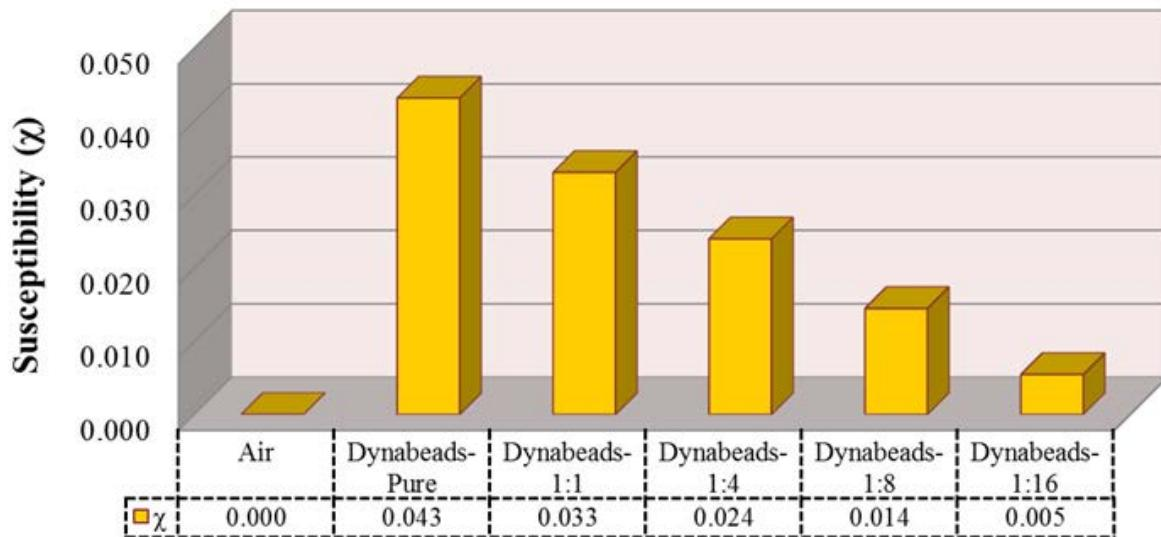
Figure 4.17 Relationship between susceptibility ( $\chi$ ) and different magnetic fluid concentrations.
