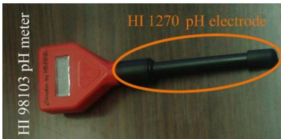
Figure 4.8 The pH meter and its pH electrode.
