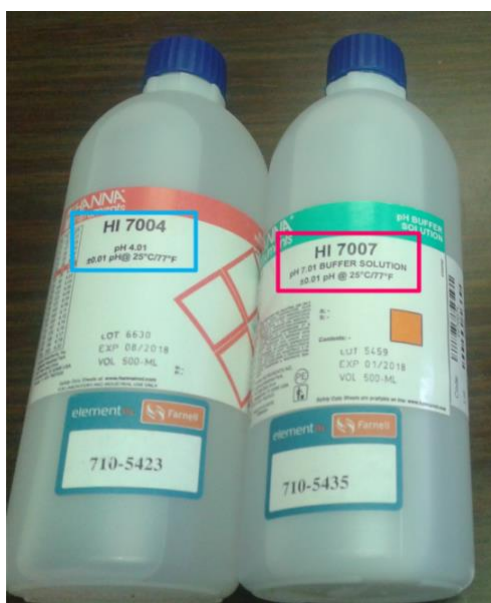
Figure 4.9 The pH 7.01 and 4.01 buffer solutions.
