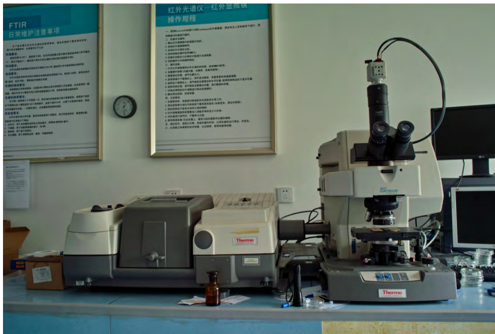
Figure 3-1. Picture of the Nicolet 5700 FTIR spectrometer coupled with a microscope located at USTC
