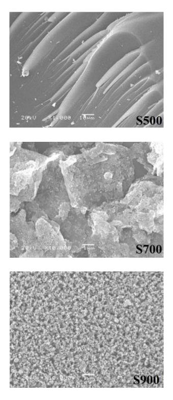
Fig. 6.1 Typical SEM images of the FePc pyrolyzed at various temperatures (S500, S700 and S900).
