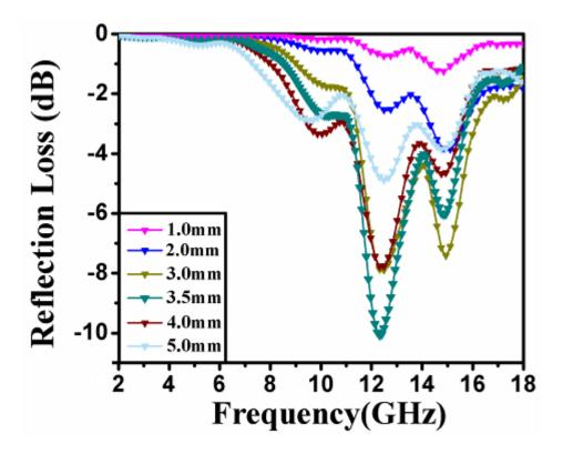
Figure 6.11 Microwave reflection loss of FePc/BPh composites
