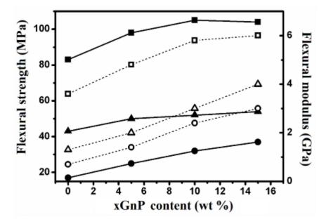
Fig. 3.6 Comparison of the flexural strength (closed symbols) and modulus (open symbols) between the xGnP/BPh (square; this work) and xGnP-15/PP (triagle; ref. [25]) and xGnP-15/HDPE (cycle; ref. [37]).
