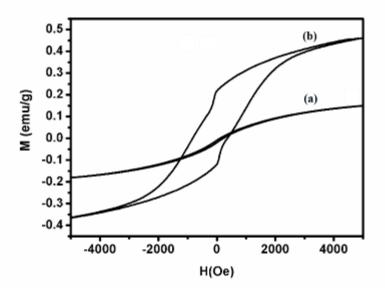
Fig. 7 Room-temperature magnetization curve of CNTs.
