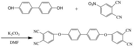
Fig. 2.1 Synthesis of BPh monomer
