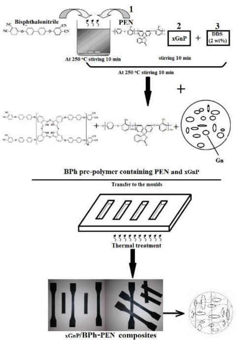
Fig. 2.5 Preparation process of xGnP/BPh nanocomposites
