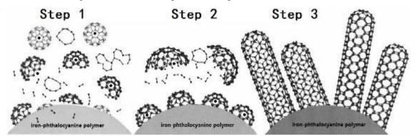
Fig. 5.3 Proposed growth mechanism of the carbon nanotubes from pyrolysis of iron phthalocyanine polymer.Step 1: the nucleation of carbon fragments starts and some of them are melted in metal particlesStep 2: the metal particles are covered with the carbon fragmentsStep 3: the carbon nanotubes start to grow at eutectic temperature.
