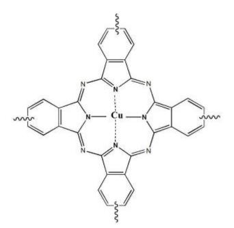
Fig. 1.4. Structure of copper phthalocyanine
