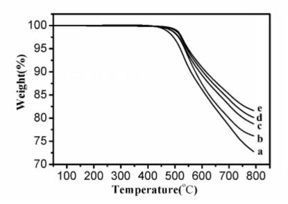
Fig. 3.3 TGA curves of the BPh polymer and xGnP/BPh nanocomposites.
