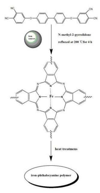
Fig. 2.6 Preparation of iron phthalocyanine polymer.
