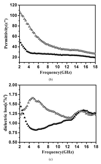
Fig. 5.7 Dielectric properties of the CNTs
