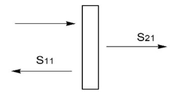
Fig. 5-6 An equivalent diagram of the free space test method
