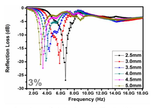
Fig. 6.9 Microwave reflection loss of S2, S3 with different layer thicknesses.
