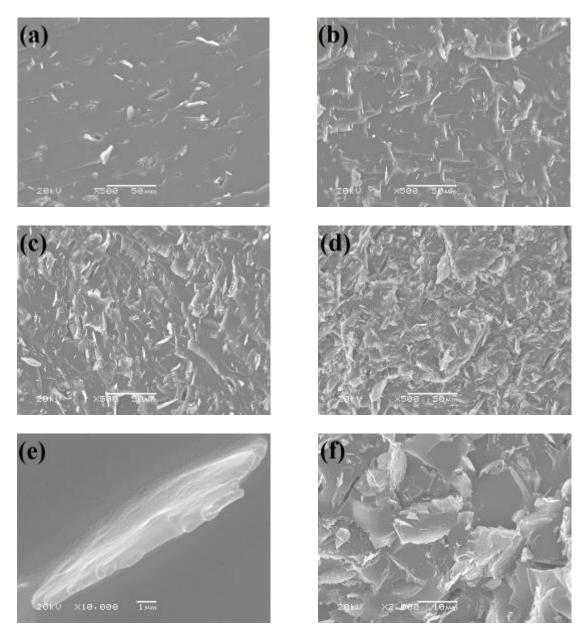
Fig. 3.5 SEM images of the fracture surfaces of xGnP/BPh naocomposite.
