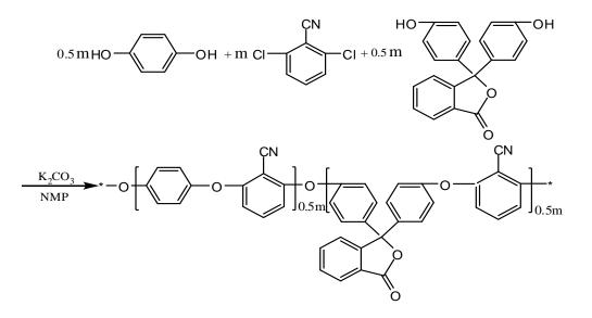
Fig. 2.3 Synthesis of phenolphthalein-based PEN copolymers
