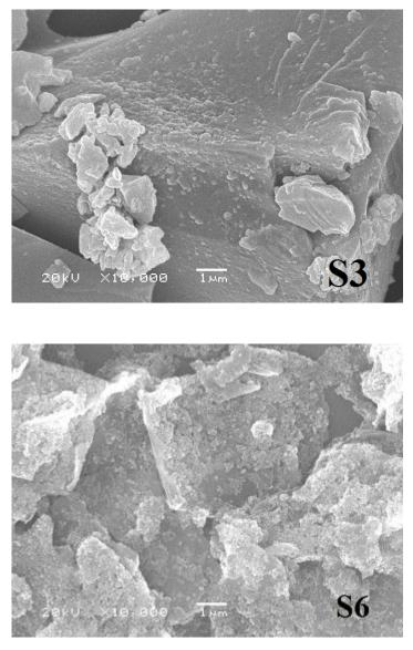
Fig. 6.6 SEM images of the FePc with different amount catalysis loading (pyrolyzed at 700 °C).
