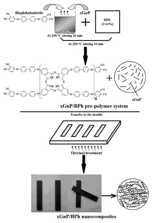
Fig. 2.2 Preparation process of xGnP/BPh nanocomposites.
