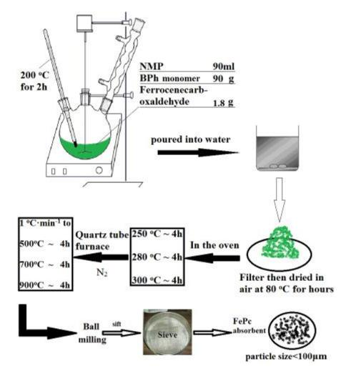
Fig. 2.6 Preparation of iron phthalocyanine absorbent.
