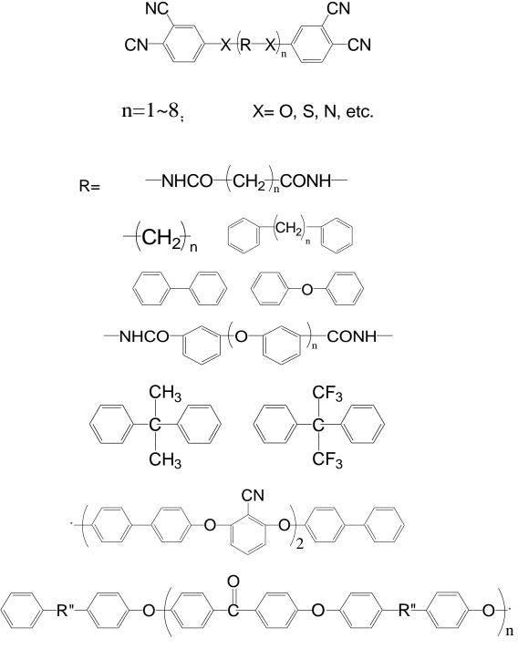
Fig. 1.5 Typical structures of phthalonitrile monomers.
