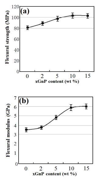
Fig. 3.4 Mechanical properties of the xGnP/BPh nanocomposites.
