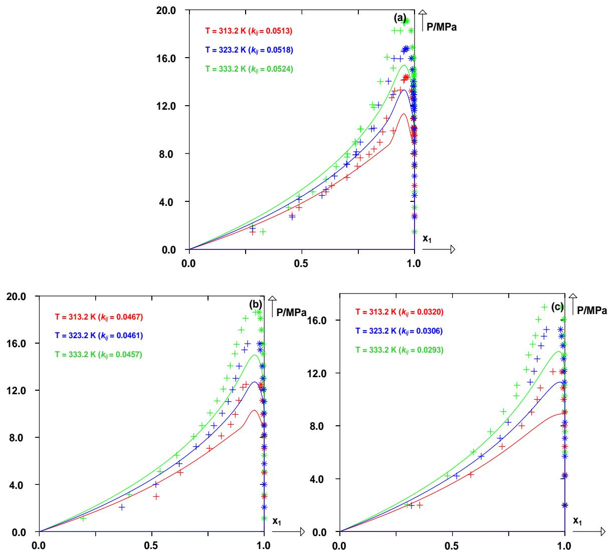
**Fig. 4 Prediction of isothermal bubble and dew curves for the binary systems containing  $\text{CO}_2$  and the C18 ethyl ester: (a):  $\text{CO}_2$  (1) + ethyl stearate (2), (b):  $\text{CO}_2$  (1) + ethyl oleate (2) and (c):  $\text{CO}_2$  (1) + ethyl linoleate (2). (+): experimental bubble points, (\*): experimental dew points and (Solid lines): predicted curves with the PPR78 model.**
