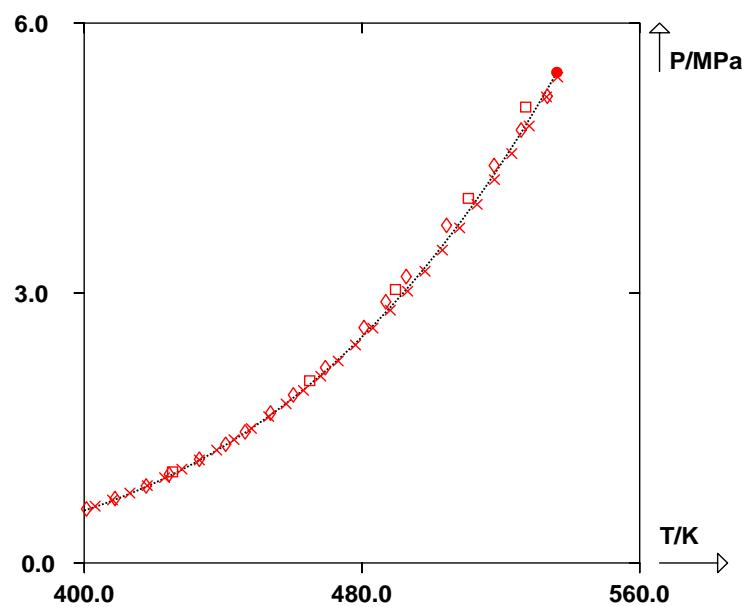
**Fig. 19 Vaporisation curve of chloroform; (□): Stull [68], (◊): Campbell and Chatterje [69], (x): Xiang [70], (Dashed lines): predicted by the PPR78 model and (●): experimental critical points [this work].**
