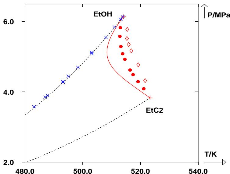
**Fig. 11** Global phase diagram of the system ethanol (1) + ethyl acetate (2) in the P-T projection. Experimental critical points: (●): this work, (◇): Hu et al. [75], (✖): saturated vapour pressures of ethanol, (+): critical points of pure components, (Solid lines): critical curve predicted by the PPR78 model and (Dashed lines): vaporisation curves predicted by the PPR78 model.
