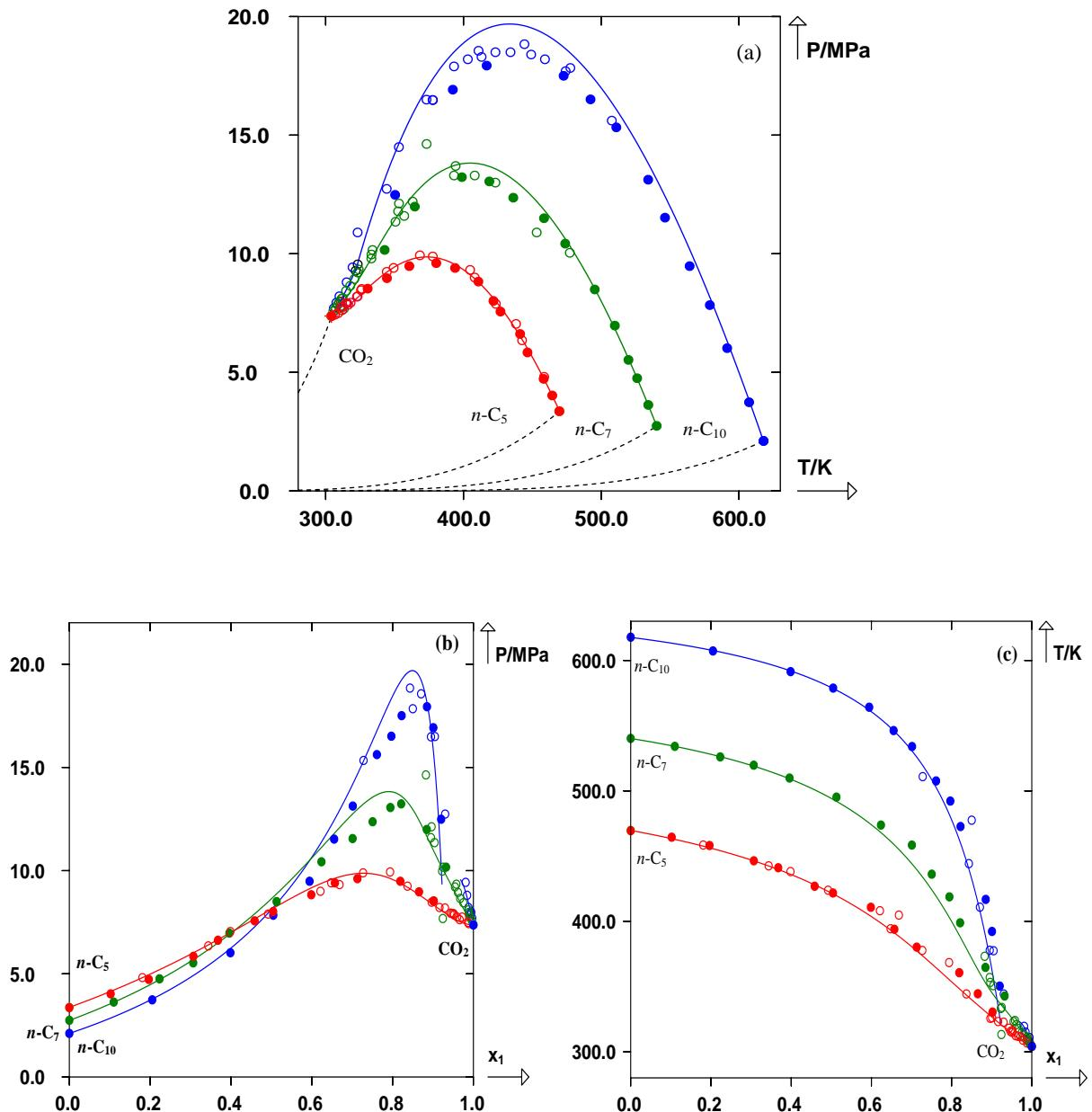
**Fig. 15** Critical loci for the systems:  $\text{CO}_2$  (1) + *n*-pentane (2),  $\text{CO}_2$  (1) + *n*-heptane (2) and  $\text{CO}_2$  (1) + *n*-decane (2) in (a)  $P$ - $T$  projection, (b)  $P$ - $x$  projection and (c)  $T$ - $x$  projection. (Solid lines): predicted curves with the PPR78 model, (dashed lines): vaporization curves of pure compounds, Experimental critical points: (●): this work and (○): literature [4-16].
