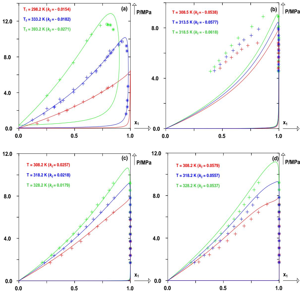
**Fig. 2 Prediction of isothermal bubble and dew curves for the binary system containing  $\text{CO}_2$  and the saturated ethyl ester; (a):  $\text{CO}_2$  (1) + ethyl acetate (2), (b):  $\text{CO}_2$  (1) + ethyl butanoate (2), (c):  $\text{CO}_2$  (1) + ethyl hexanoate (2) and (d):  $\text{CO}_2$  (1) + ethyl octanoate (2). (+): experimental bubble points, (\*): experimental dew points, (○): experimental critical points and (Solid lines): predicted curves with the PPR78 model.**
