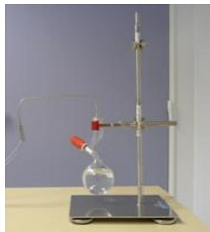
**Fig. 3 Experimental setup for degassing a liquid compound.**
