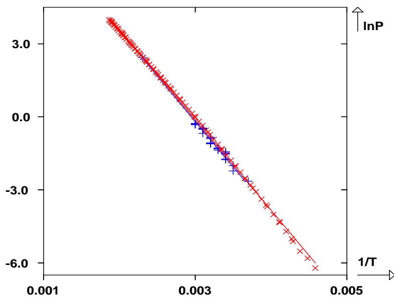
**Fig. 17 Vapour pressures and azeotropic pressures available in literature for the binary system acetone (1) + chloroform (2); (x): Vapour pressures [68-70], (+): Azeotropic pressures [49-57, 59-63] and (Solid lines): linear regressions**
