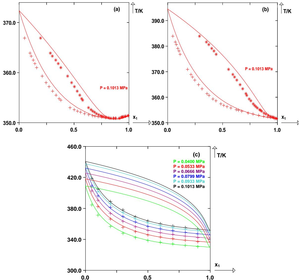
**Fig. 9 Prediction of isobaric bubble and dew curves for the binary system containing ethanol and the saturated ethyl ester at different pressures; (a): ethanol (1) + ethyl propionate (2), (b): ethanol (1) + ethyl butanoate (2) and (c): ethanol (1) + ethyl hexanoate (2). (+): experimental bubble points, (\*): experimental dew points and (Solid lines): predicted curves with the PPR78 model.**
