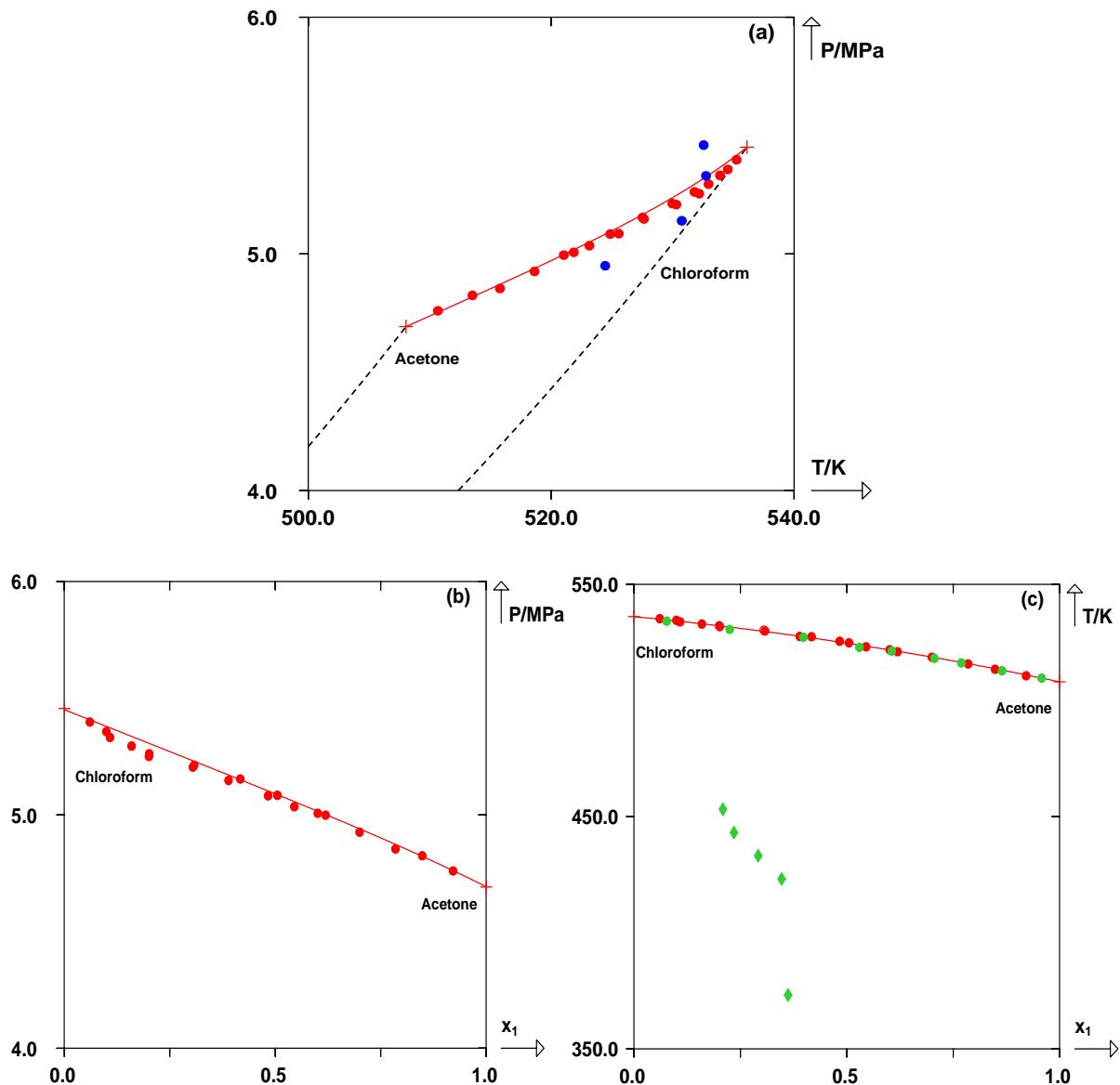
**Fig. 18 Critical locus for the system acetone (1) + chloroform (2) in (a): P-T projection, (b) P-x projection and (c): T-x projection. (Solid line): critical locus correlated by the PPR78 model, (Dashed lines): vaporization curves of pure compounds predicted by the PPR78 model, Experimental critical points; (●): this work, (●): Kuenen and Robson [67], (●): Campbell and Musbally [58]. Azeotropic Compositions; (◆): Campbell and Musbally [58].**
