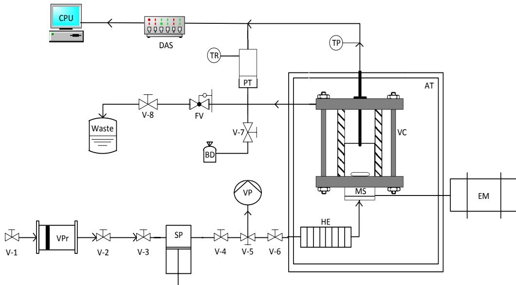
**Fig. 2 Schematic diagram of the apparatus; PS: Pressurized source, VPr: Volumetric press, SP: Syringe pump, CB: Cryostat bath, VP: Vacuum pump, HE: Heat exchanger, EM: Electric motor, MS: Magnetic stirrer, VC: View cell, AT: Air thermostat bath (oven), TP: Platinum resistance temperature probe, PT: Pressure transducer, TR: Temperature regulator, BD: Bursting disc, FV: Flow regulation valve, DAS: Data acquisition system, CPU: Central processor unit and V: Valve.**
