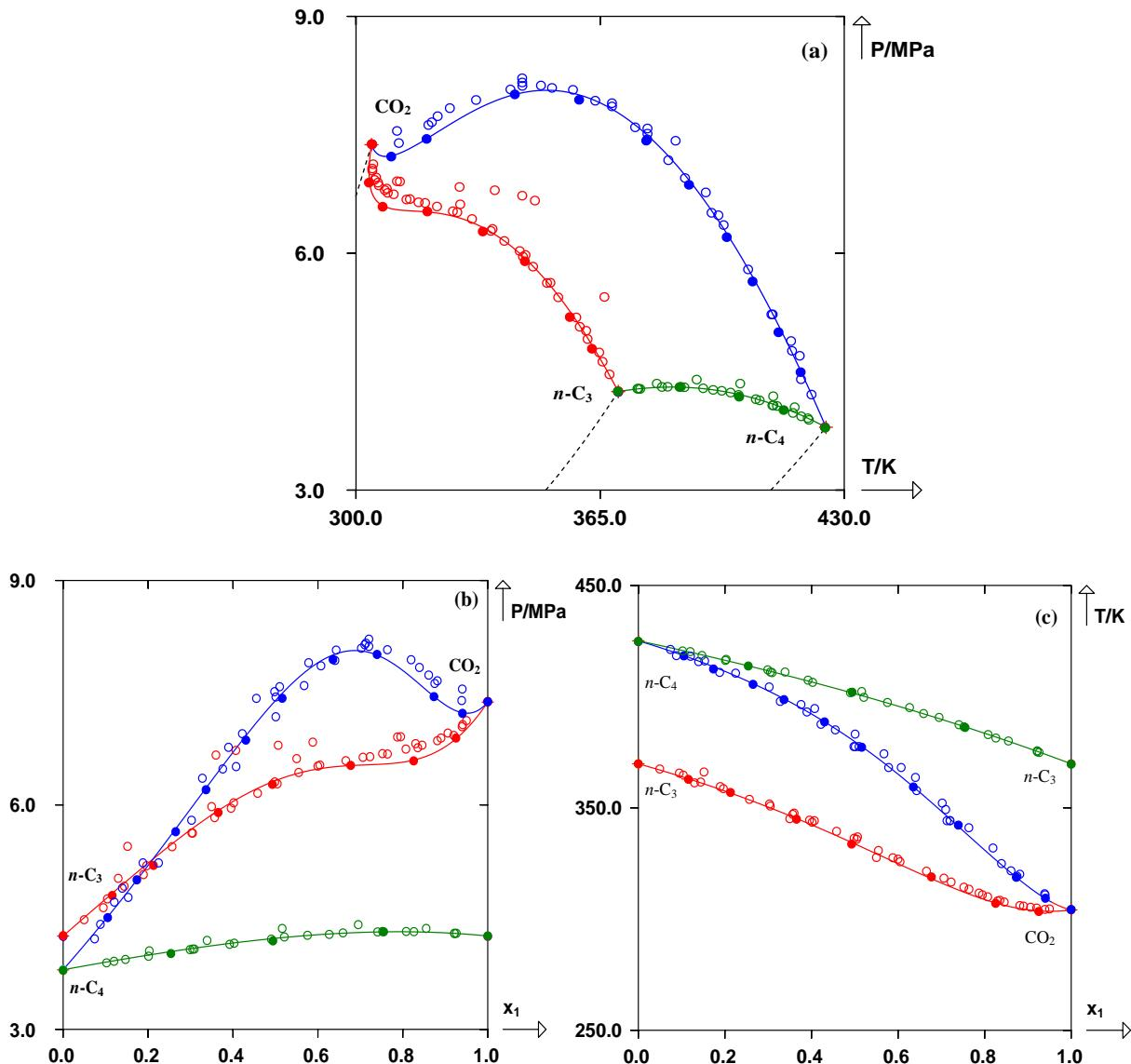
**Fig. 16 Critical loci for the systems:  $\text{CO}_2$  (1) + *n*-propane (2),  $\text{CO}_2$  (1) + *n*-butane (2) and *n*-propane (1) + *n*-butane (2) in (a)  $P$ - $T$  projection, (b)  $P$ - $x$  projection and (c)  $T$ - $x$  projection. (Solid lines): predicted curves with the PPR78 model, (dashed lines): vaporization curves of pure compounds, Experimental critical points: (●): this work and (○): literature [19-31].**
