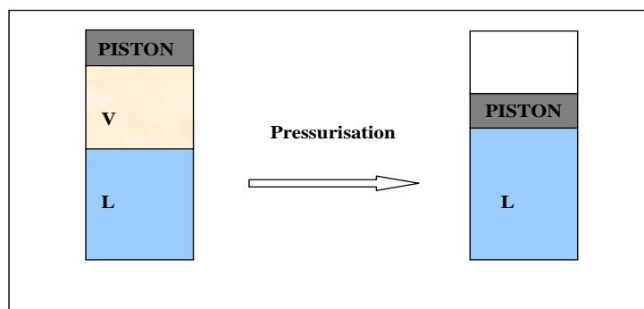
**Fig. 7 Schematic diagram of the pressurisation process.**
