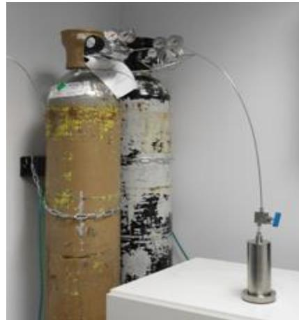
**Fig. 5 Transfer of a gas compound from a gas cylinder to the volumetric press.**
