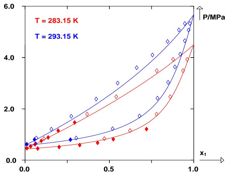
**Fig. 16 Isothermal bubble and dew curves for the system CO<sub>2</sub> (1) + R1234yf (2) at two temperatures; Experimental bubble and dew points at 283.15 K : (◊): This work, (♦): Di Nicola et al. [153], Experimental bubble and dew points at 293.15 K: (◊): This work, (♦): Di Nicola et al. [153] and (Solid line): bubble and dew curves correlated by the PPR78 model.**
