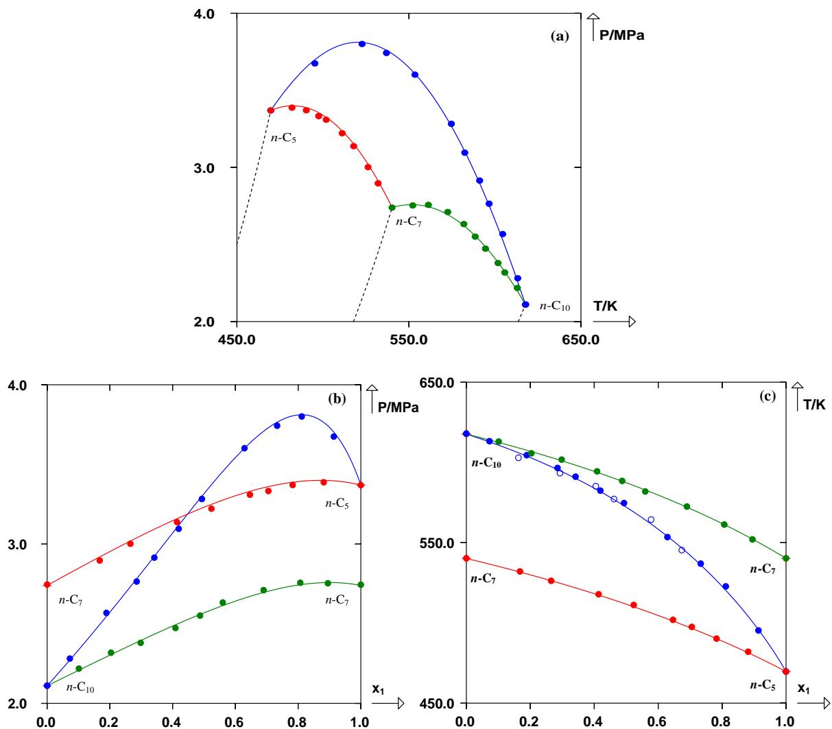
**Fig. 14 Critical locus for the systems: *n*-pentane (1) + *n*-heptane (2), *n*-pentane (1) + *n*-decane (2) and *n*-heptane (1) + *n*-decane (2) in (a) *P-T* projection, (b) *P-x* projection and (c) *T-x* projection. (Solid lines): predicted curves with the PPR78 model, (dashed lines): vaporization curves of pure components, Experimental critical points: (●): this work and (○): Hicks and Young [11].**
