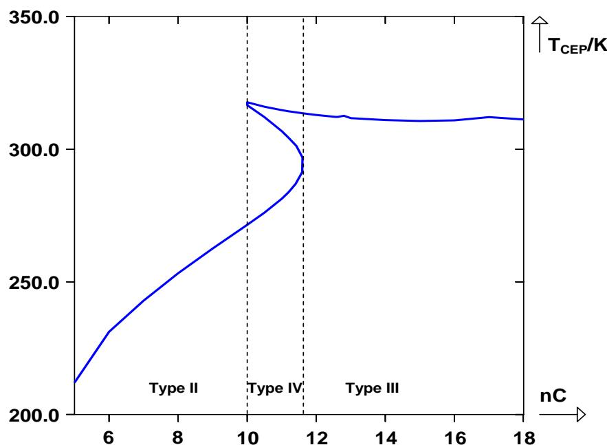
**Fig. 7 Evolution of phase behaviour type for the systems involving CO<sub>2</sub> and saturated ethyl ester in the homologous series (from ethyl pentanoate to ethyl stearate)**
