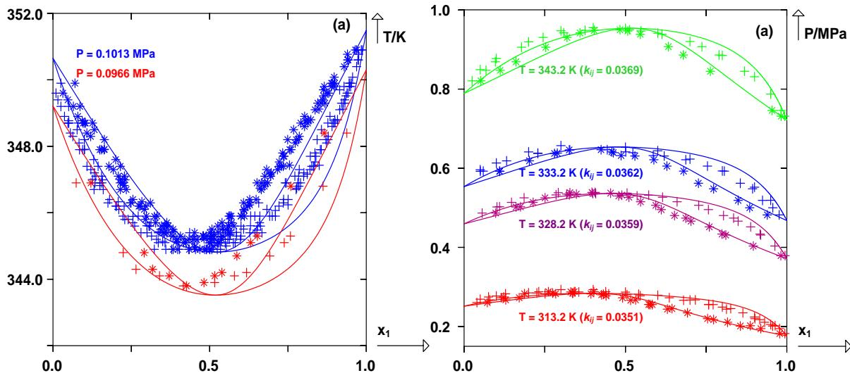
**Fig. 8 Prediction of bubble and dew curves of the system ethanol (1) + ethyl acetate (2); (a): isobaric diagram and (b): isothermal diagram. (+): experimental bubble points, (\*): experimental dew points and (Solid lines): predicted curves with the PPR78 model.**
