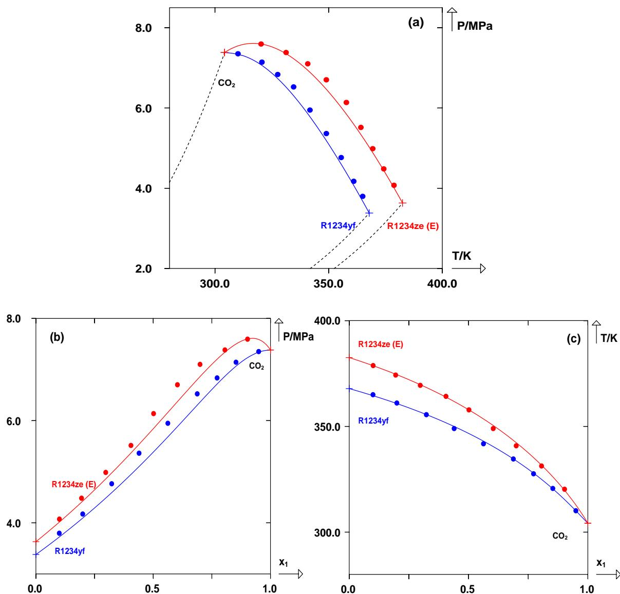
**Fig. 17 Critical loci for the systems  $\text{CO}_2$  (1) + R1234yf (2) and  $\text{CO}_2$  (1) + R1234ze (E) (2) shown in (a): P-T diagram, (b): P-x diagram and (c): T-x diagram. (Closed symbol): experimental critical points, (+): critical points of the pure substances, (Solid line): correlated results by the PPR78 model and (Dashed line): vaporisation curves of pure components.**
