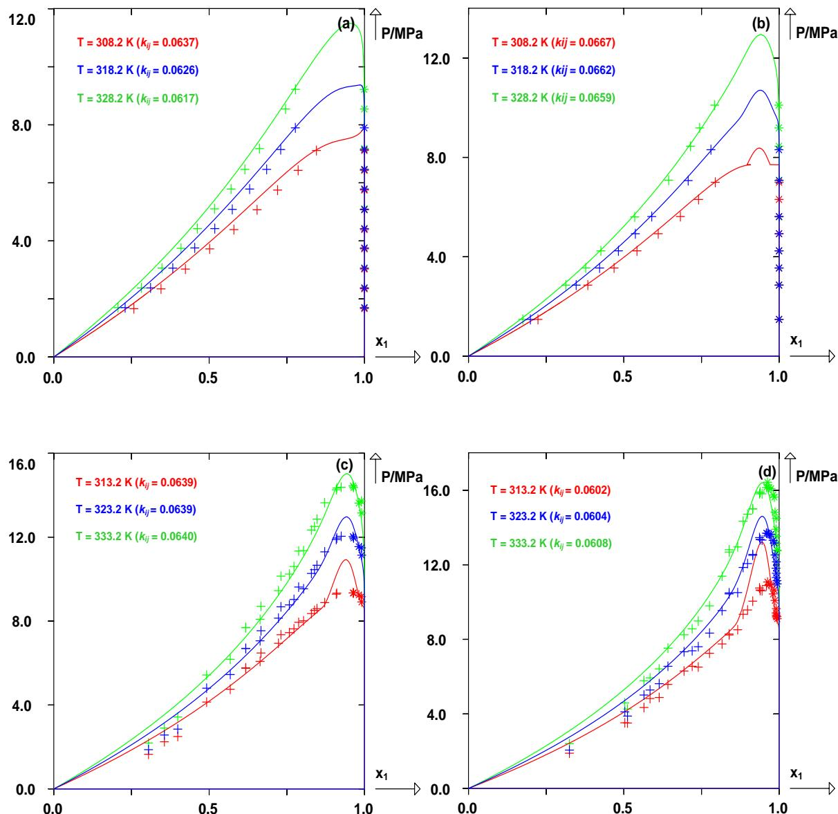
**Fig. 3 Prediction of isothermal bubble and dew curves for the binary system containing  $\text{CO}_2$  and the saturated ethyl ester; (a):  $\text{CO}_2$  (1) + ethyl decanoate (2), (b):  $\text{CO}_2$  (1) + ethyl laurate (2), (c):  $\text{CO}_2$  (1) + ethyl myristate (2) and (d):  $\text{CO}_2$  (1) + ethyl palmitate (2). (+): experimental bubble points, (\*): experimental dew points, and (Solid lines): predicted curves with the PPR78 model.**
