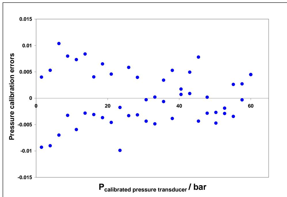
**Fig. 11** Pressure calibration errors: the difference between pressures measured using the calibrated pressure transducer and those measured using the pressure transducer (available in our experiments) correlated one.
