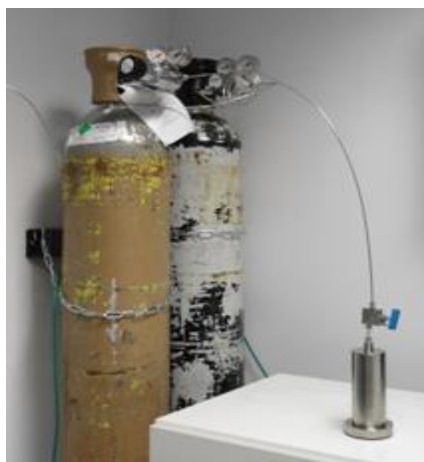
Fig. 5 Transfer of a gas compound from a gas cylinder to the volumetric press.
