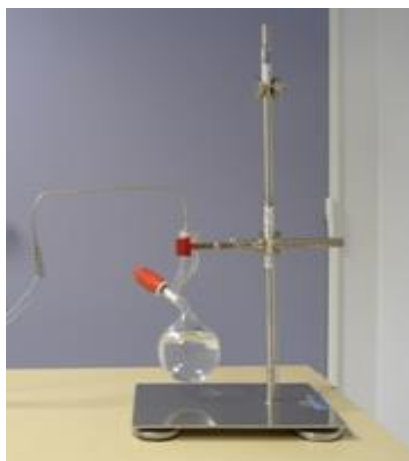
Fig. 3 Experimental setup for degassing a liquid compound.
