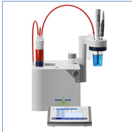
Figure 35. Banc de titration Mettler Toledo T50
