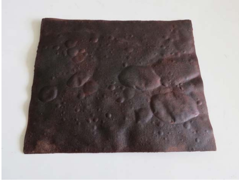
Figure 1 10-ply impregnated papers at 10% moisture content pressed at 180 °C temperature at 60 kg/cm 2 pressure for 240 s. Note the unacceptable bubbles on the laminate surface
