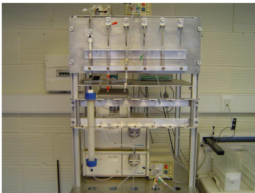
Figure 11. Flash Chromatography apparatus (robot).
