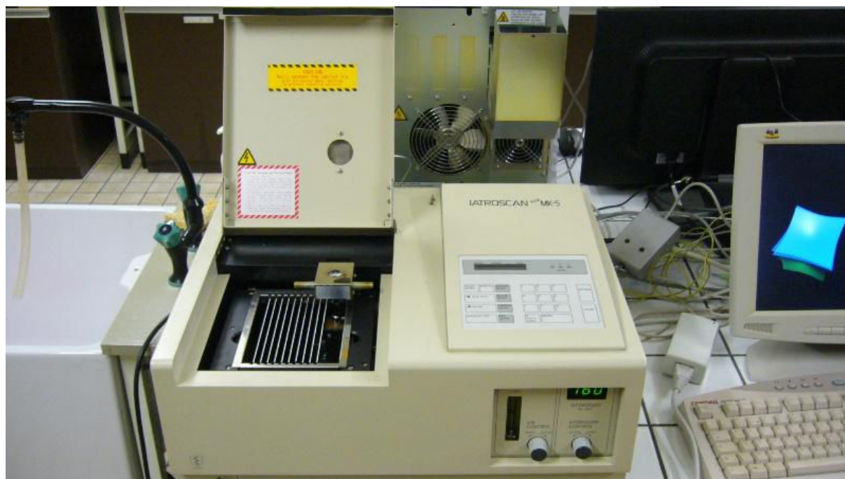
Figure 17. Iatroscan TLC-FID MK V for lipid classes
