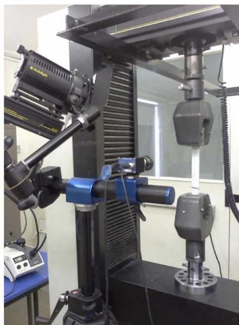
Fig. 3. DIC technique applied to provide micro-scale information.
