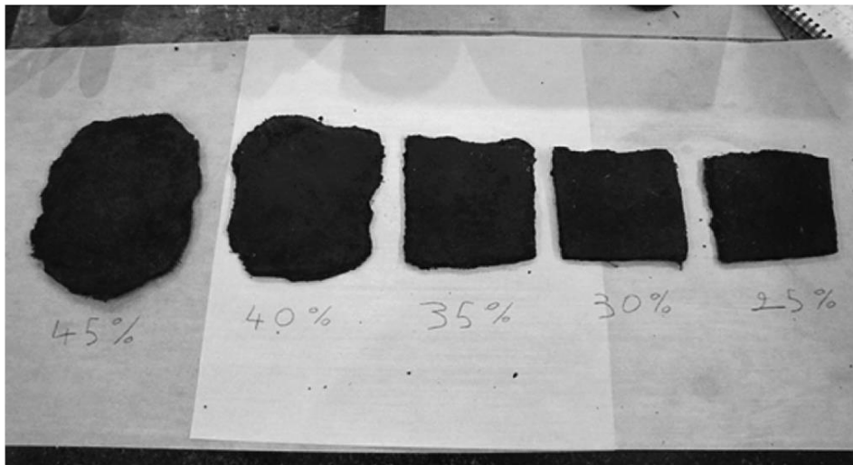
Figure 2. Mat expansion during pressing, respectively at 45, 40, 35, 30 and 25% MC before pressing.
