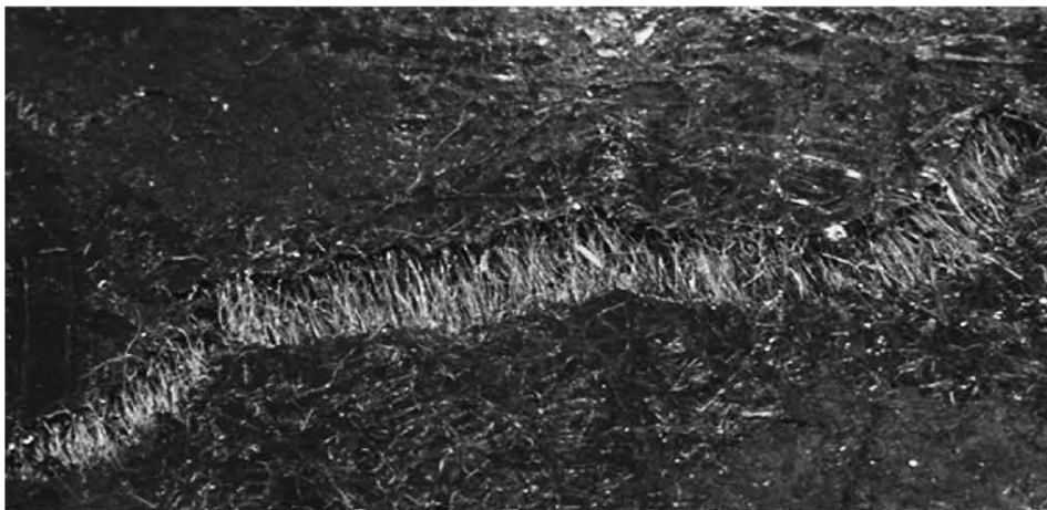
Figure 5. Crack occurring during the pressing of larger panels. Regular fiber orientation indicates that this phenomenon appears in the early time of pressing, when the core resin is still soft.
