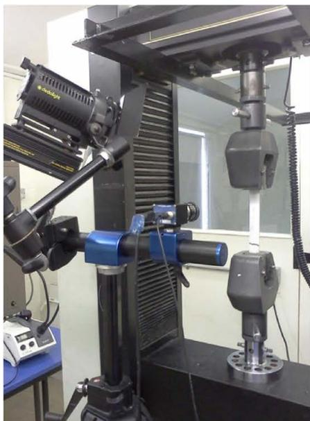
Fig. 3. DIC technique applied to provide micro-scale information.
