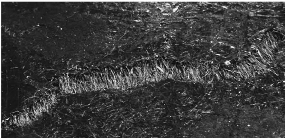
**Figure 5.** Crack occurring during the pressing of larger panels. Regular fiber orientation indicates that this phenomenon appears in the early time of pressing, when the core resin is still soft.
