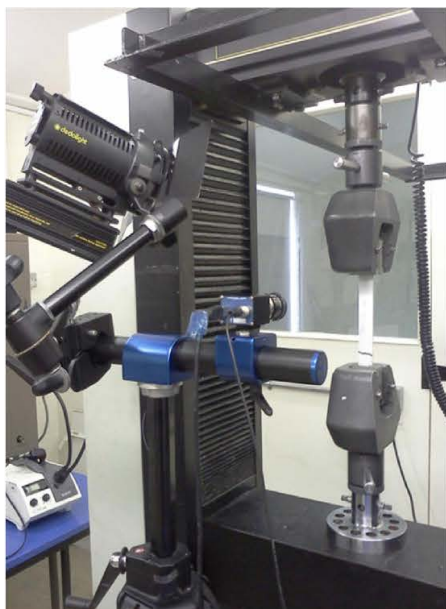
Fig. 3. DIC technique applied to provide micro-scale information.
