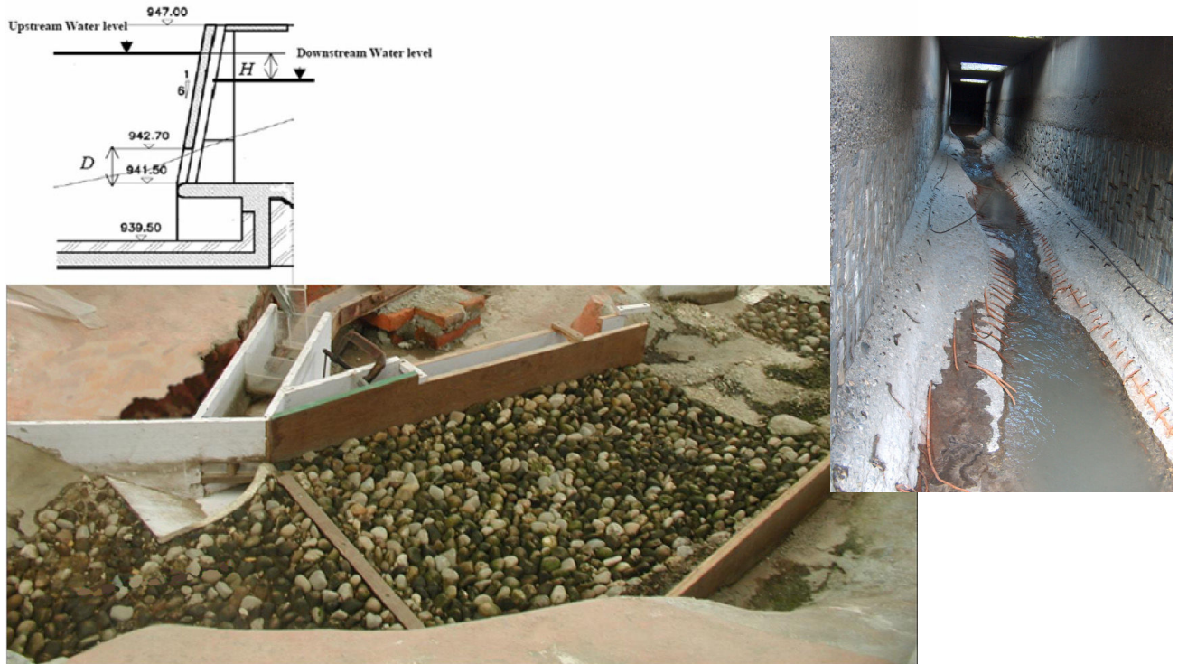
Figure B2: Experimental pre-design of the intake setting (Shrestha and Phuyal, 2006) that display the present gate setting within the intake wall: two upper intake gate and, below them, an undersluice gate at the end of a bed load hopper wall. Right picture = view of the boulder evacuation channel just downstream the boulder undersluice gate.
