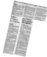
(a) A skewed document image : the skew angle is equal to 12^\circ
